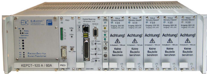
Fig. 5: Crate with five switched-mode power supplies, one of them being redundant (courtesy of J. Eckoldt, DESY)
