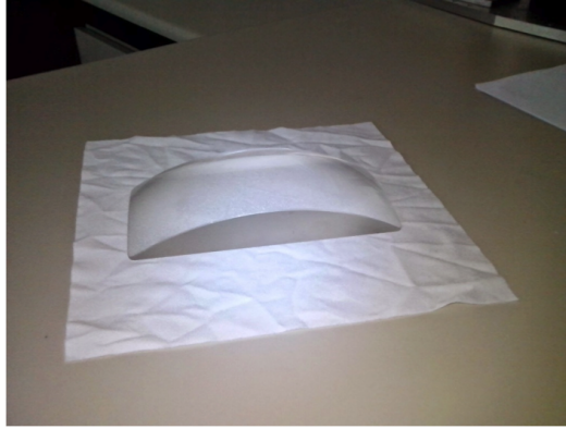
Figure 1: The lens used in the testbeam.
