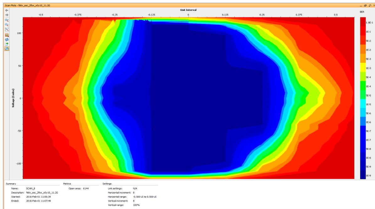
Eye diagram of tested link from LDPB to gFEX
