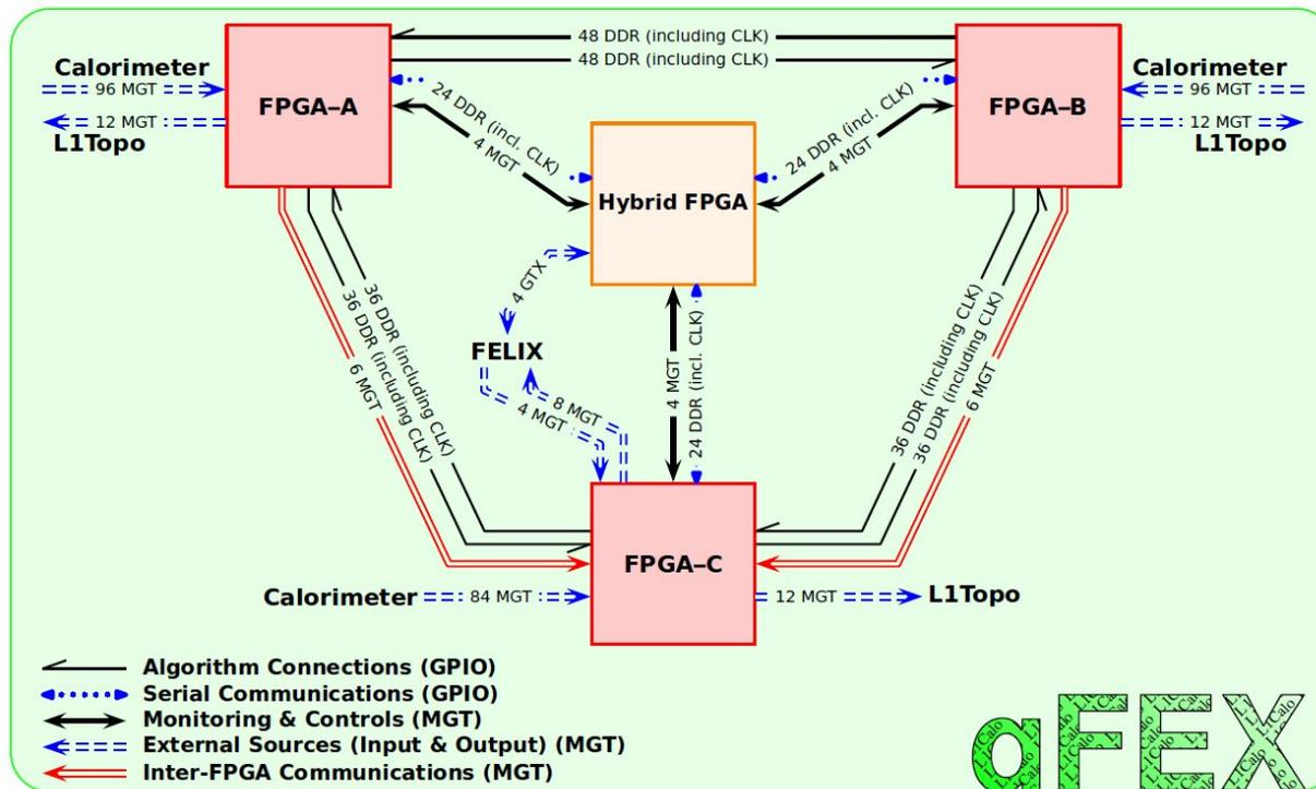
Block diagram of gFEX Prototype
