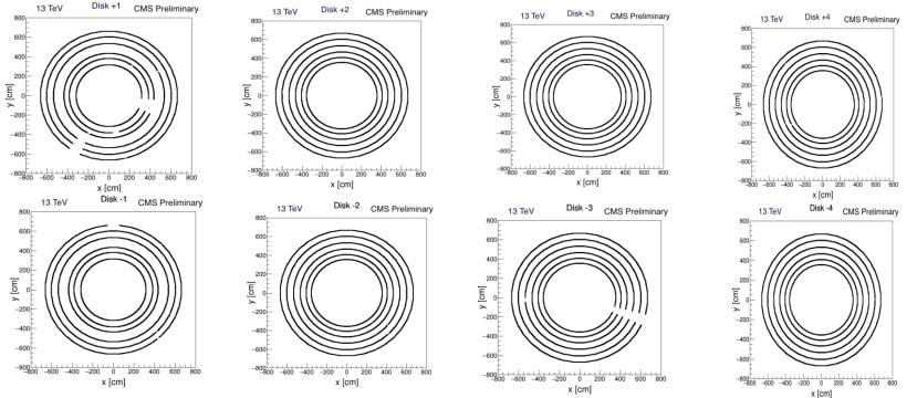
The plots represent the cross-sectional view of the  $1^{st}$ ,  $2^{nd}$ ,  $3^{rd}$  and newly installed  $4^{th}$  positive and negative RPC stations in the forward regions of the CMS (Endcaps). The black points show the position of the reconstructed hits in the middle of the strips. The results are based on the analysis of the collision data taken since September 2015 to the end of the year at sqrt (s) =13 TeV at 3.8T. The empty spots correspond to the inactive signal electrodes.
