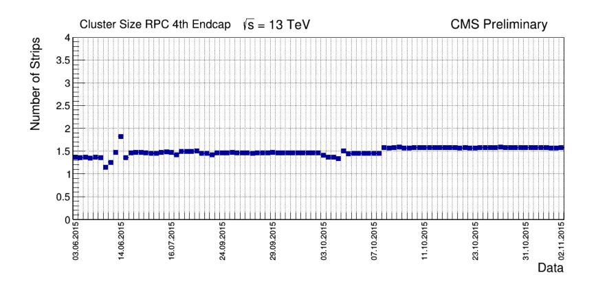
The plot represents the history of the Mean Cluster Size for the newly installed RPC chambers on the 4-th Endcap stations. The fluctuation in the middle of June are due to the performed HV scan. The fluctuations in the beginning of October are due to the performed threshold scan. The details about the expected values of cluster size can be found (CERN/LHC 97-32 (https://web.physik.rwth-aachen.de/~hebbeker/cms\_muon\_tdr.pdf)).
