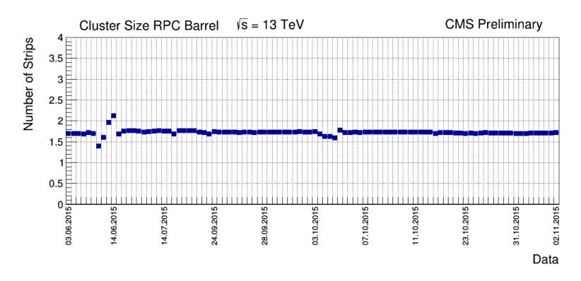
The plot represents the history of the Mean Cluster Size for the Barrel for the 2015 physics data taking. The fluctuation in the middle of June are due to the performed HV scan. The fluctuations in the beginning of October are due to the performed threshold scan. The details about the expected values of cluster size can be found (CERN/LHC 97-32 (https://web.physik.rwth-aachen.de/~hebbeker/cms\_muon\_tdr.pdf)).
