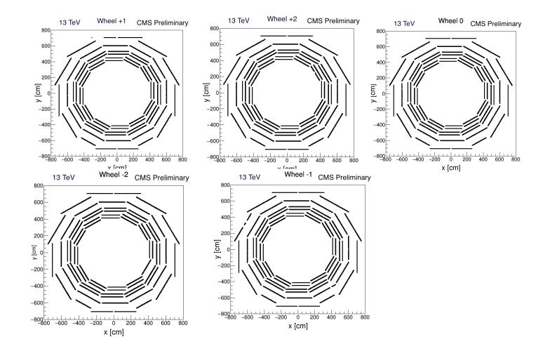
The plots represent the cross-sectional view of the barrel wheels of the RPC system. The black points show the position of the reconstructed hits in the middle of the strips. The results are based on the analysis of the collision data taken since September 2015 to the end of the year at sqrt (s) =13 TeV at 3.8T. The empty spots correspond to the inactive signal electrodes.
