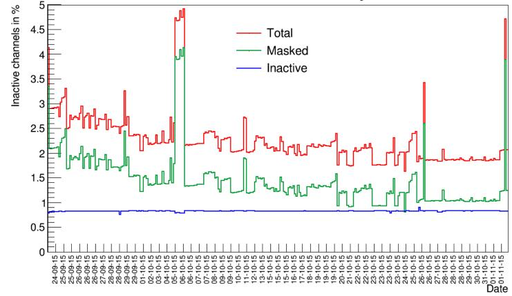
The plot represents the fraction of channels not operational during 2015. The blue line represents the number of inactive (non responsive) channels, while the number of the masked strips (green line) changes with a time as they are adjusted per run depending on the performance of the system. The observed peaks related to the bigger number of masked strips caused by the temporary hardware problems, which were successfully resolved.
