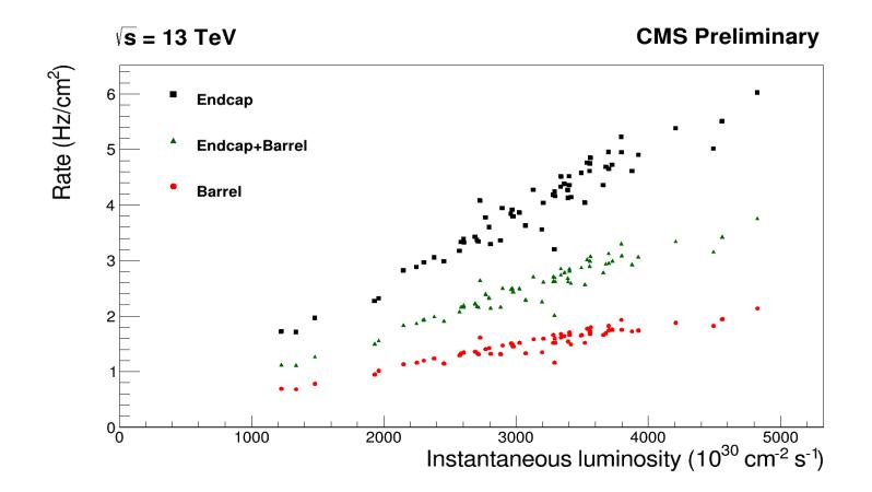
The plot shows the average hit rate vs. instantaneous luminosity, with 2015 13 TeV p-p collisions data. The red dots represent the rate measured in Barrel and the black represent the rate measured in Endcap. The green markers relate to the overall rate evaluated for the entire RPC system.
