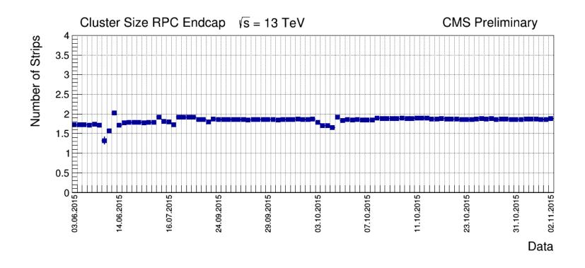
The plot represents the history of the Mean Cluster Size for the Endcap for the 2015 physics data taking. The fluctuation in the middle of June are due to the performed HV scan. The fluctuations in the beginning of October are due to the performed threshold scan. The details about the expected values of cluster size can be found (CERN/LHC 97-32 (https://web.physik.rwth-aachen.de/~hebbeker/cms\_muon\_tdr.pdf)).
