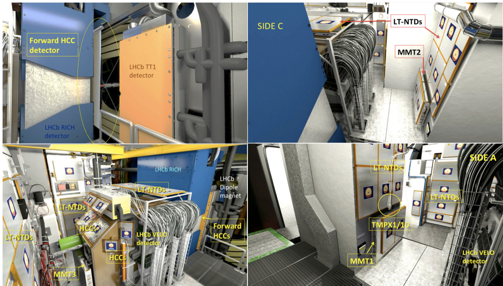
Figure 2. Views of a visualization of the MoEDAL detector showing elements of all 4 sub-detector systems
