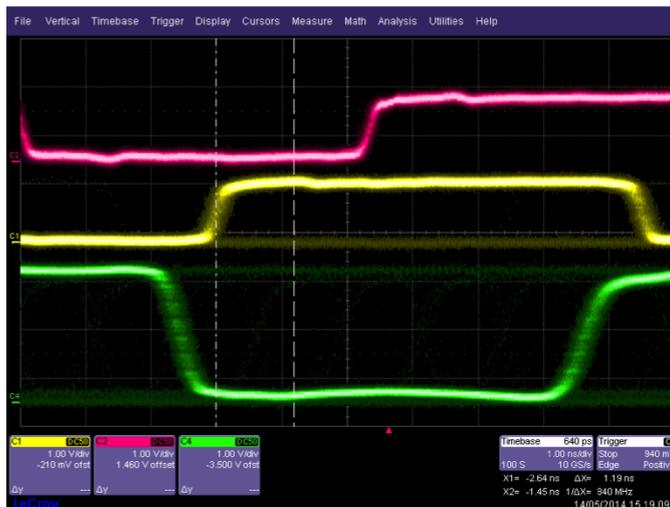
**Figure 7.** Deterministic latency feature of NaNet<sup>3</sup> SerDes: the plot scope shows the phase alignment of the transmitting (purple) and receiving (yellow) parallel clocks after 12 h test of periodic reset and initialisation sequence.
