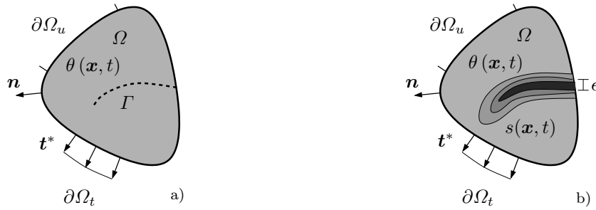
Fig. 1 Body with internal discontinuities (sharp cracks) \Gamma a), and approximation of internal discontinuities by a phase field s(\mathbf{x}, t) b).
