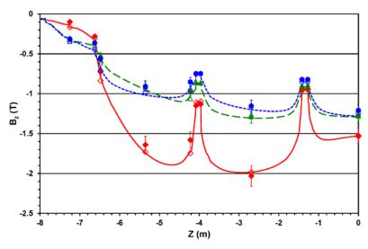
**Fig. 4** Axial magnetic flux density measured (filled markers) and calculated (opened markers) in the first (rhombs), second (triangles), and third (circles) barrel layers vs. Z-coordinate at the operational current of 18.164 kA. The lines represent the calculated values along the Hall sensors locations at the negative X-coordinates and at the Y-coordinates of –4.805 (solid line), –5.66 (dashed line), and –6.685 (dotted line) m, corresponded to the first, second, and third barrel layer blocks
