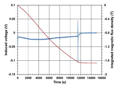
**Fig. 2** Induced voltage (left scale, noisy curve) and the integrated average magnetic flux density (right scale, smooth curve) in the tail catcher block cross-section at Z=0 m and at the operational current of 18.164 kA. The rapid maximum and minimum voltage at 11445 s corresponds to the transition from the standard discharge to the fast discharge of the magnet
