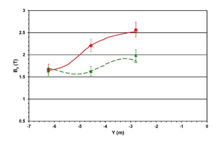
**Fig. 5** Axial magnetic flux density measured (filled markers) and calculated (opened markers) in the first (rhombs) and second (triangles) end-cap disks vs. Y-coordinate at the operational current of 18.164 kA. The lines represent the calculated values in the middle planes of the end-cap disks
