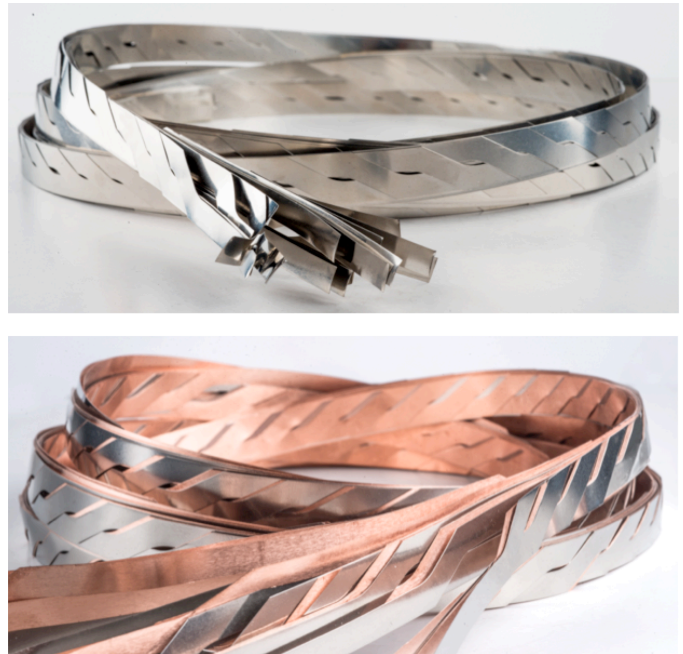
Fig. 6. Samples of Roebel dummy cables produced within the scope of the EuCARD2 activities: SS tape (top) and assembly of SS and Cu tapes
