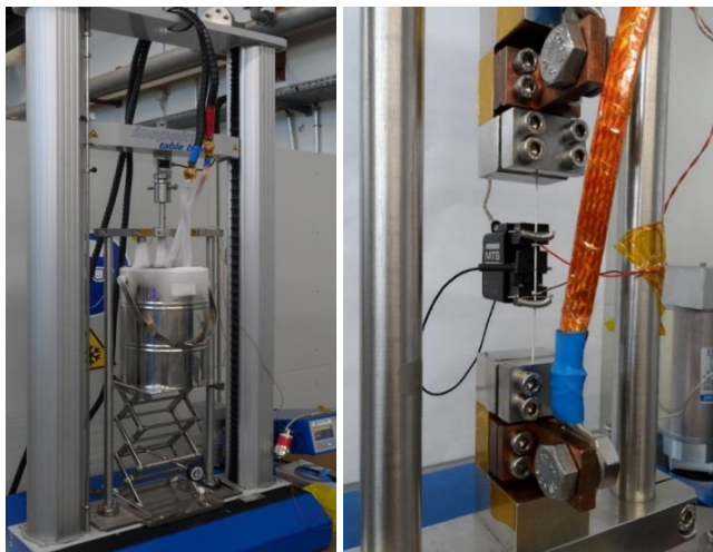
Fig. 2. (a) UTM equipped for I_c vs stress and strain measurements in liquid nitrogen. (b) Bi-2212 wire mounted in the grips instrumented with voltage taps, clip on extensometer and current leads.
