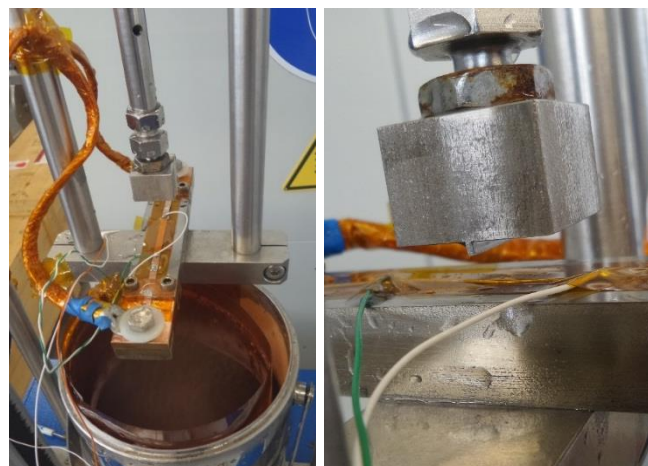
Fig. 3. (a) UTM with sample holder and pressing tool for I_c vs transverse compressive stress measurements. (b) Detailed view of the 1 mm-wide pressing tool.
