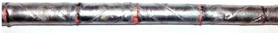
Figure 2. Five tapered sections of the CORC cable, each 17 mm in length, held together by a bandage of solder.
