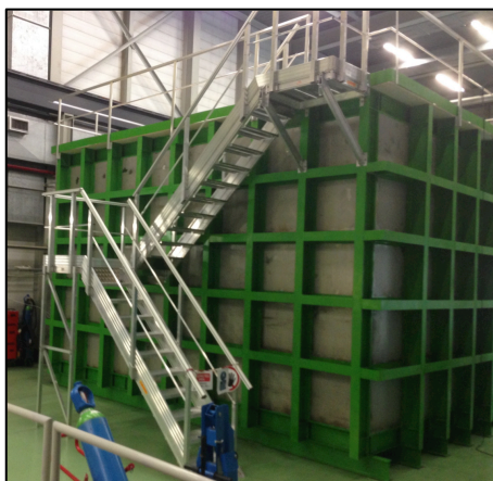
Figure 3. Photo of the WA105 1x1x3 outer support structure.
