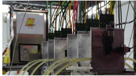
Figure 7: The telescope composed of six silicon planes.
