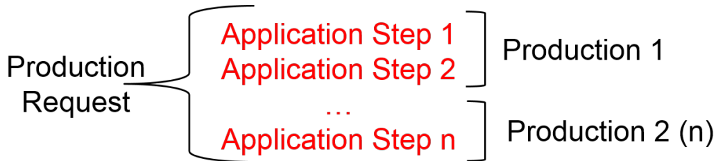
Figure 5: Concepts of a Production Request: each request is composed by a number of steps. Steps are grouped and run by productions.
