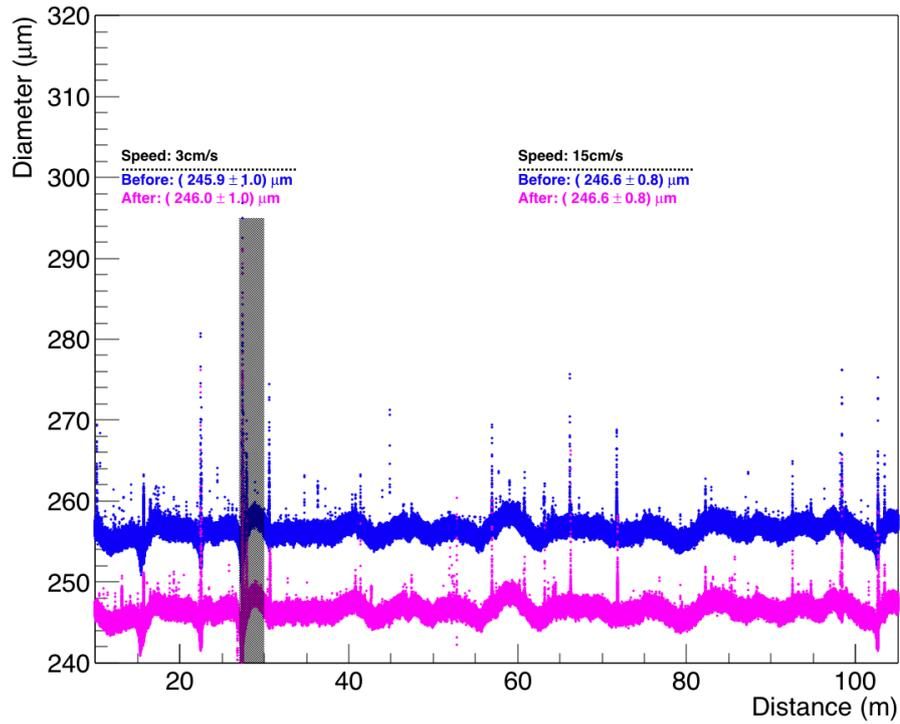
Figure 5: Fibre diameter measurement before (blue) and after (magenta) running the fibre through the hot tool at low and medium speed. The blue curve has been shifted up by 10 ( $\mu\text{m}$ ) for better clarity. Mean values and RMS are essentially unaffected.
