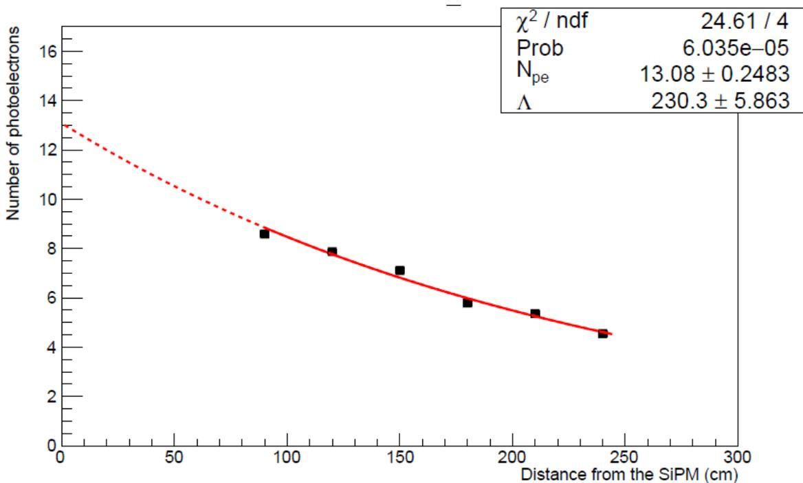
Figure 3: Light yield versus distance from the Sr-90 source for fibre CE160229-1 after passing through the hot tool at a speed of 3 cm/s. The light yield extrapolated to  $d = 0$  results in 13.1 photoelectrons.
