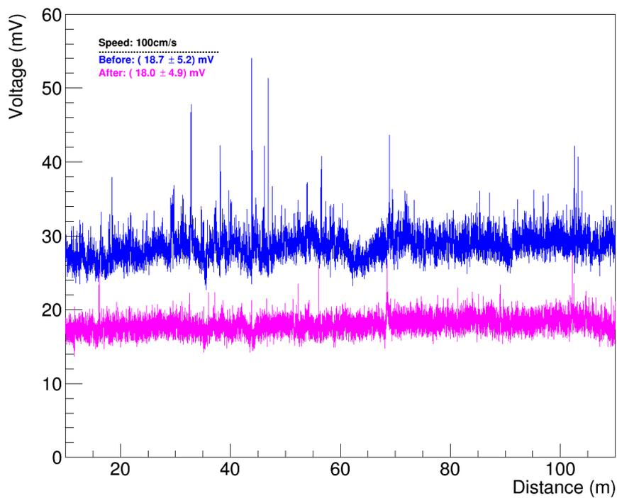
Figure 6: Cladding test signal versus fibre position for high speed passage of the hot tool. As above, the blue curve is shifted up by 10 mV. The measurement 'after' (magenta) has a slightly lower average and RMS.
