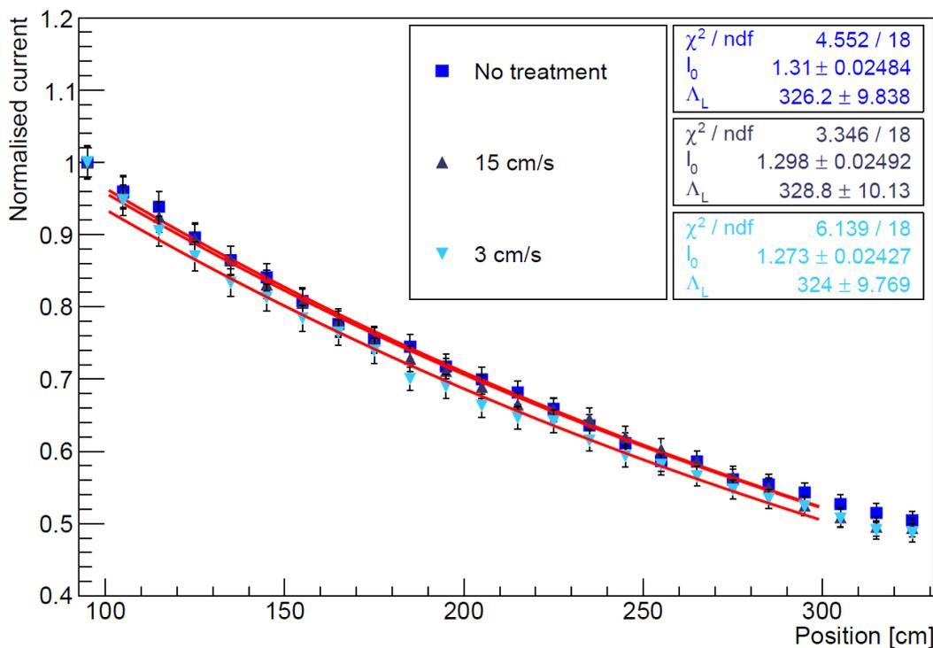
Figure 2: Averaged light attenuation of the three investigated fibre sets. The attenuation length  $\Lambda_L$  is determined by a single exponential fit to the data between 100 and 300 cm from the photodetector. The three data sets refer to the untreated fibres and the two drawing speeds of 3 and 15 cm/s. All three sets show identical values around 325 cm.
