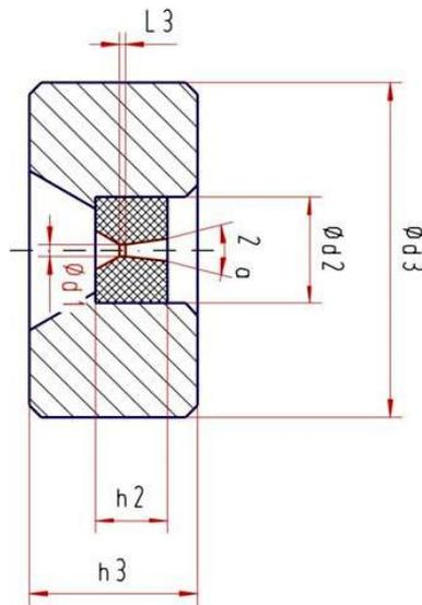
Figure 1: Geometry of the drawing tool. The drawing direction is from right to left.
