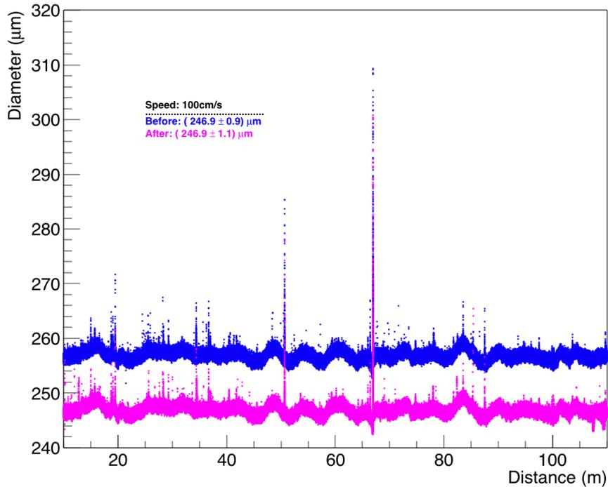
Figure 7: Fibre diameter measurement before (blue) and after (magenta) running the fibre through the hot tool at high speed. Mean value and RMS are very similar.
