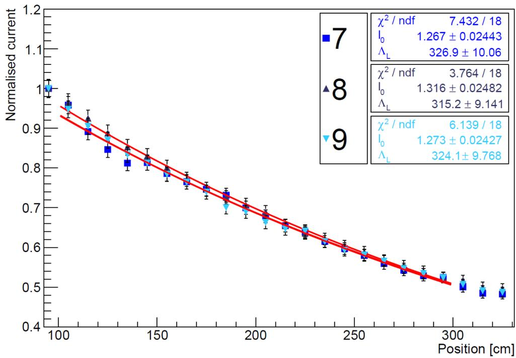
Figure 9: Light attenuation measured for the individual fibre samples. Sample 1-3 were not pulled through the tool. Samples 4-6 were pulled through the hot tool at a speed of 15 cm/s. Samples 7-9 were pulled through the hot tool at a speed of 3 cm/s.
