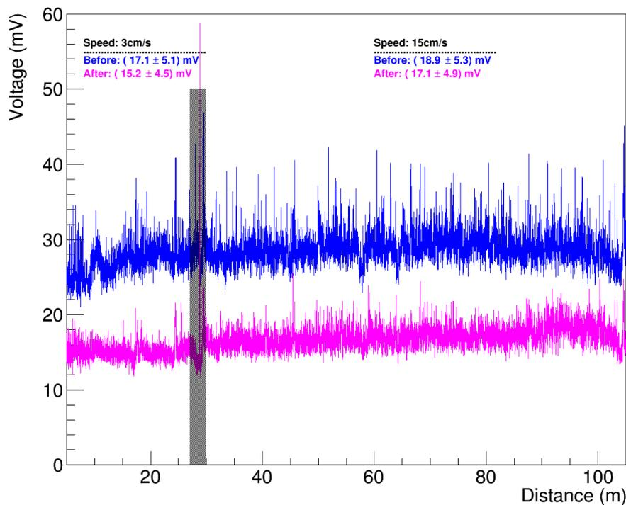
Figure 4: Cladding test signal versus fibre position for slow and medium speed passage of the hot tool. The blue curve, taken before the passage through the drawing tool, was shifted up by 10 mV for better clarity. The magenta curve was obtained after the passage. The grey bar indicates the transition from low (3 cm/s) to medium (15 cm/s) drawing speed.
