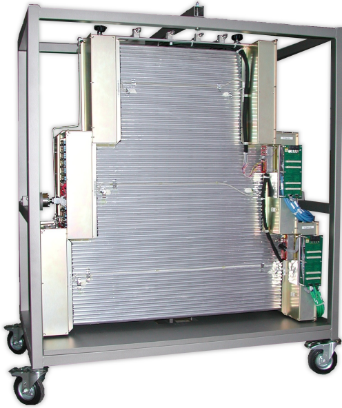
Figure 2: The sMDT prototype chamber of a size of one square meter.
