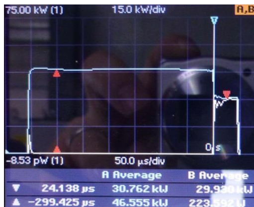
Figure 6: No amplifier shutdown with 21 cm extension.
