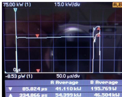
Figure 5: A discharge leads to amplifier shutdown.
