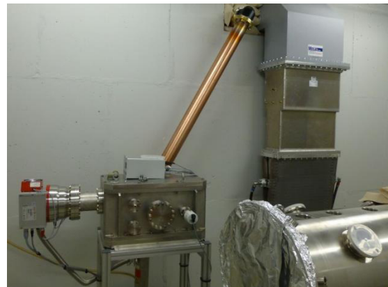
Figure 3: 325 MHz test cavity structure on support.
