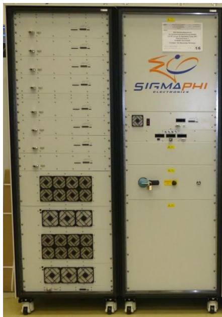
Figure 1: One of the 45 kW amplifiers.
