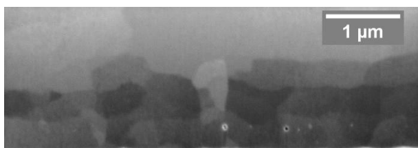
Figure 3: A layered structure of i4 sample close to the copper interface. The rare presence of nm size pores was observed.
