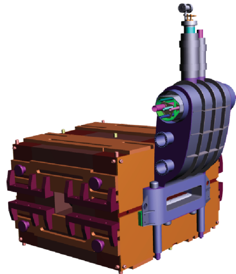
Figure 2: Outer shape of the dipole (design status 12-2014). One clearly sees the warm iron and the embedded cryostat. The big turret is due to the DN400 flange for the cryogenic and electrical interfaces standardized for ease of connection with the cryogenic jumper lines.
