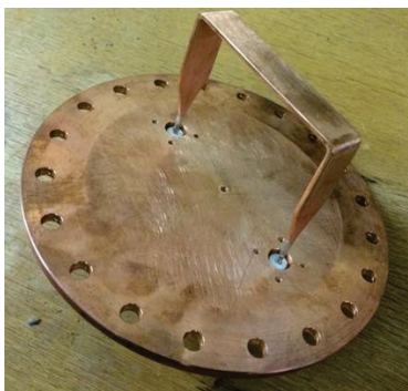
Figure 4: Example of mode coupler geometry mounted on a copper flange.
