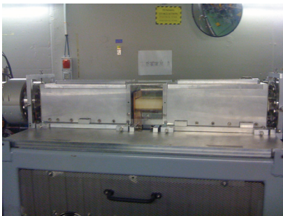
Figure 1: Vertical (left) and horizontal (right) pinger magnet installed at ALBA during summer 2014. The ceramic chamber (in white) is visible between the two structures used for the vertical (left) and horizontal (right) excitations.
