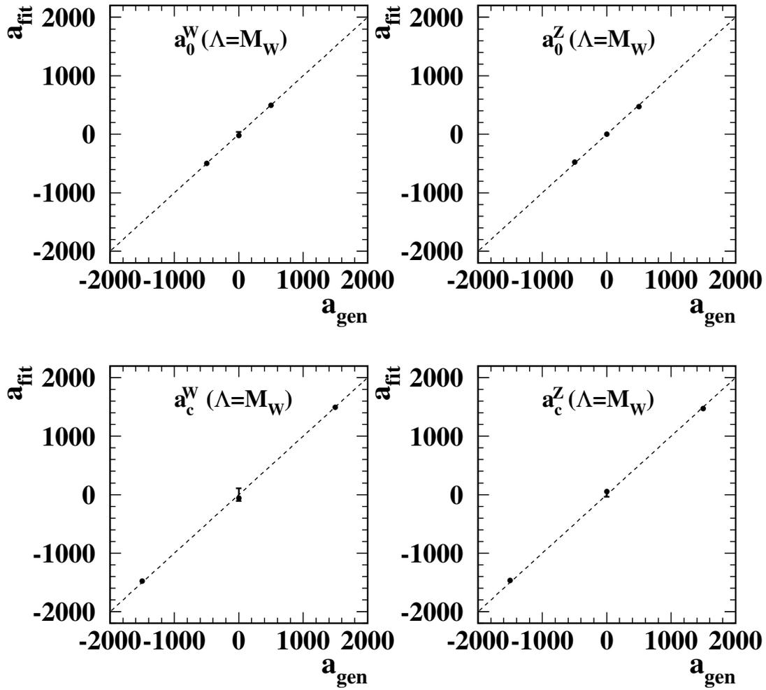
Figure 4.1: Bias test results. For each of the four couplings, the value of the parameter extracted from the fit,  $a_{\text{fit}}$ , is plotted against the coupling value with which the input sample was generated,  $a_{\text{gen}}$ . The 95% confidence level error bars are drawn.
