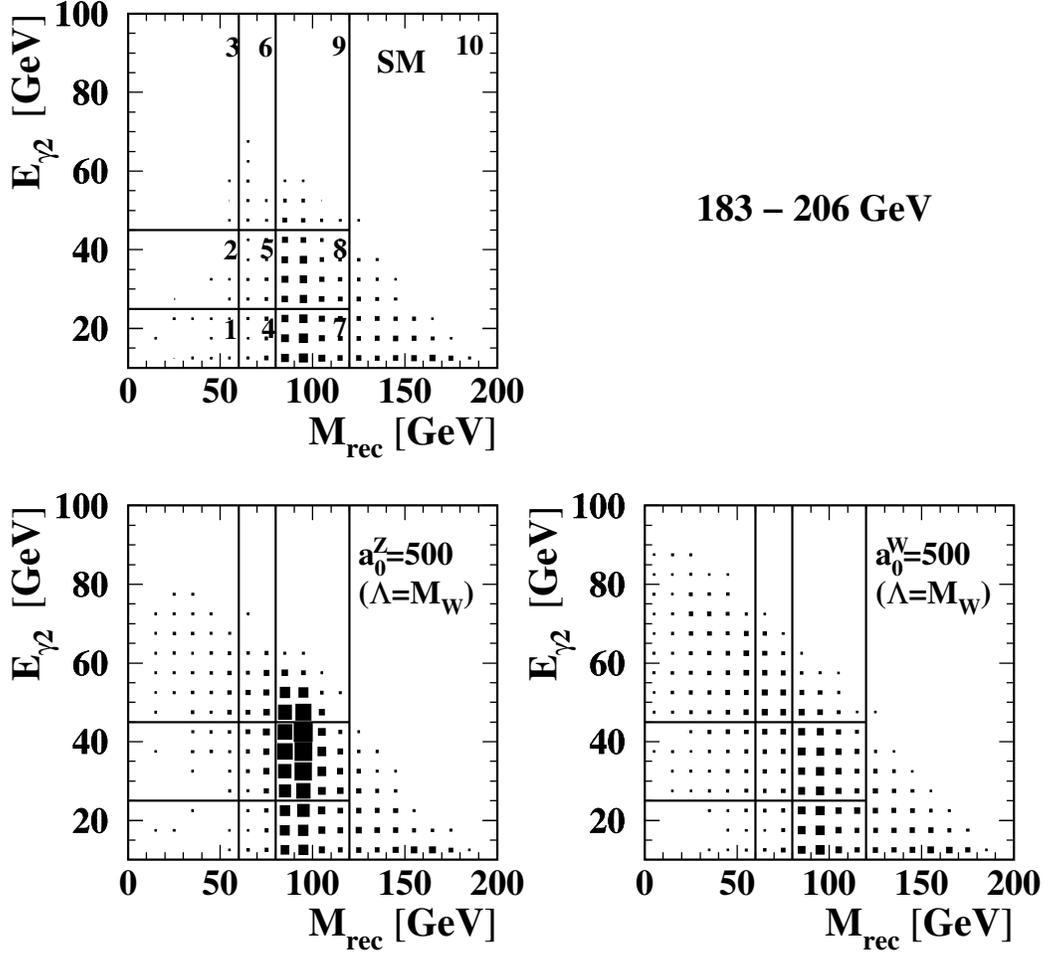
Figure 3.5: The optimal binning of  $(M_{\text{rec}}, E_{\gamma 2})$  superimposed on the expected shapes of the two-dimensional distribution in the Standard Model and anomalous  $WW\gamma\gamma$  and  $ZZ\gamma\gamma$  quartic coupling scenarios. The AQC distributions have been normalised to the Standard Model expectation.
