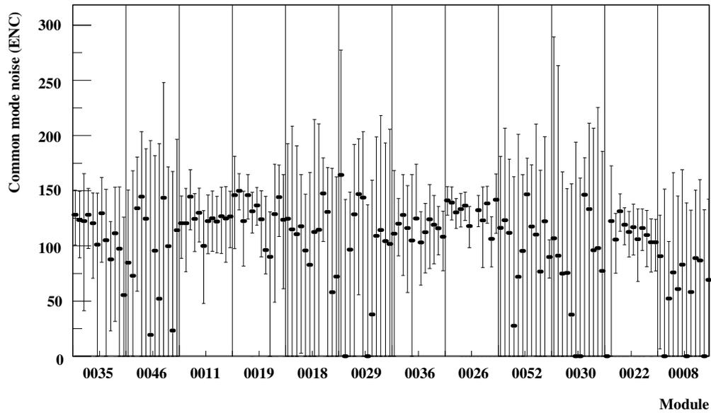
Figure 5.20: The common-mode noise values in ENC by chip for 12 modules operated on the sector. The module names are given on the  $x$ -axis: the 12 points per module correspond to the chip averaged values.
