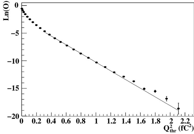
Figure 5.9: The typical  $\ln$ -occupancy versus  $Q_{\text{thr}}^2$  behaviour of one chip. The ABCD chips are not designed to be operated with their threshold set close to zero. It is concluded that no deviations from the linear dependence, which would indicate non-Gaussian noise pick-up, are seen.
