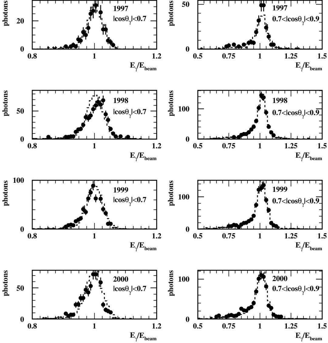
Figure 3.6: Photon energy distributions normalised to the beam energy in the barrel ( $|\cos(\theta_\gamma)| < 0.7$ ) and end-cap ( $0.7 < |\cos(\theta_\gamma)| < 0.9$ ) regions of the detector, in the four years of interest. The points with error bars show the OPAL data and the dashed histograms represent the fully simulated RADCOR Monte Carlo events.
