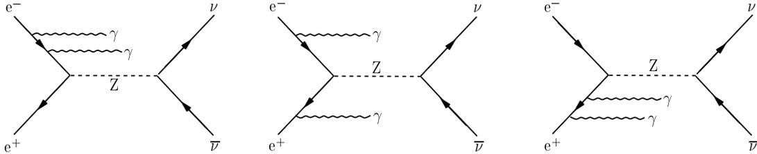
Figure 1.7: The Standard Model doubly-radiative return processes leading to  $\nu\bar{\nu}\gamma\gamma$ .
