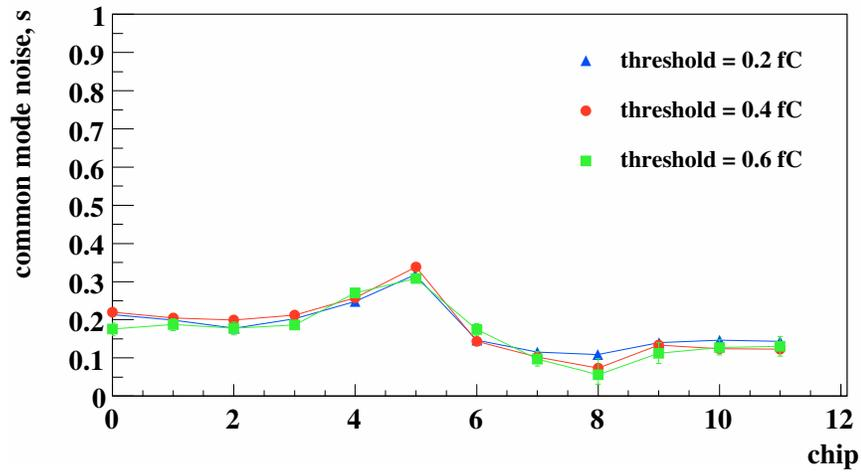
Figure 5.18: Common-mode noise by chip from the correlation method at 0.2, 0.4, 0.6 fC threshold.
