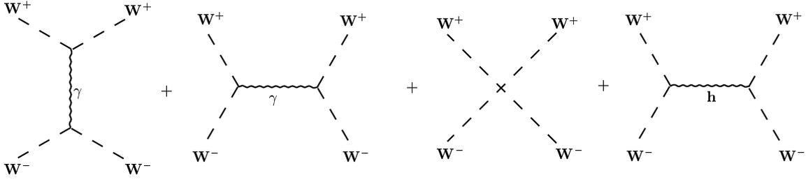
Figure 1.6: Contributions to the  $W^+W^-$ -scattering process,  $W^+W^- \rightarrow W^+W^-$ . The addition of the QGC process to the first two diagrams is not sufficient to conserve unitarity: the Higgs particle (h) exchange diagram is also required.
