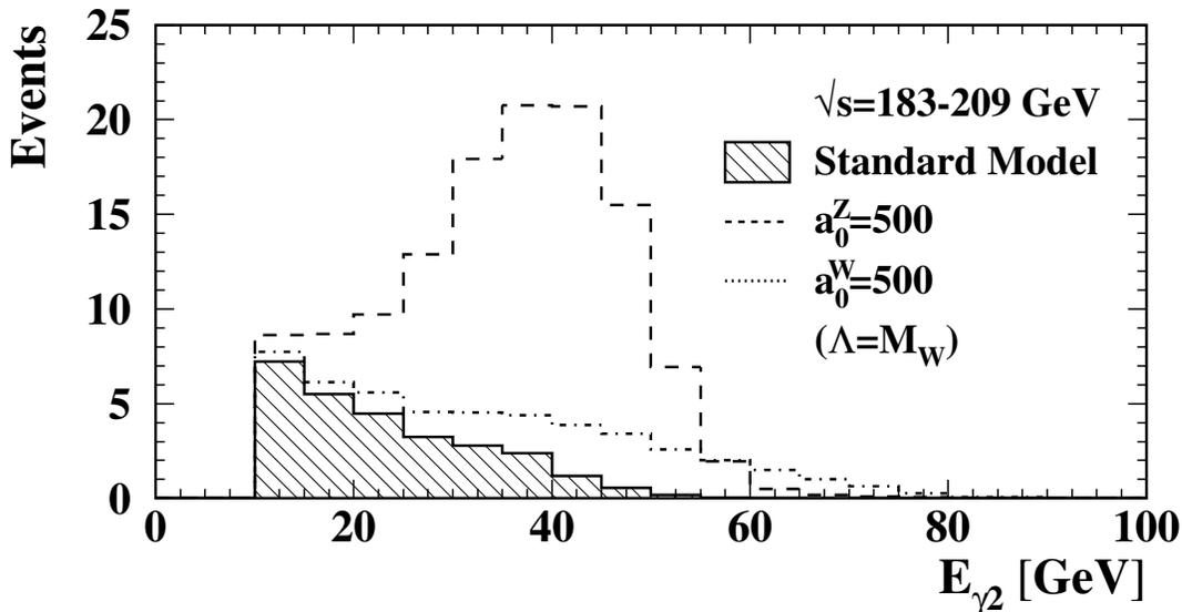
Figure 3.3: The distributions of the second highest reconstructed photon energy for the accepted  $\nu\bar{\nu}\gamma\gamma$  events, in the Standard Model and with possible  $WW\gamma\gamma$  and  $ZZ\gamma\gamma$  anomalous couplings.
