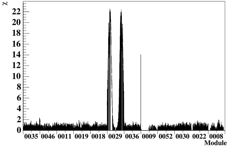
Figure 5.12: The quantity  $\chi$  of equation 5.1 plotted for all channels. Real hits were generated in module 0029. The results are consistent with there being no cross talk.
