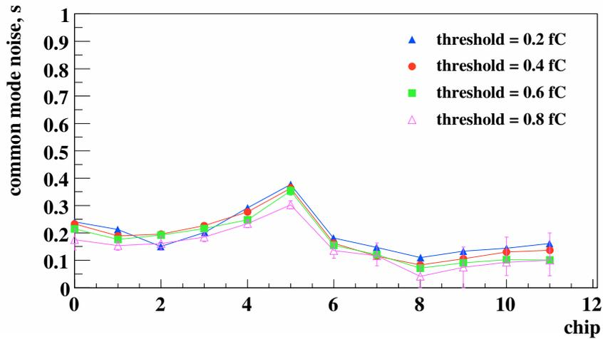
Figure 5.19: Common-mode noise by chip from the  $\Omega$  method at 0.2, 0.4, 0.6, 0.8 fC threshold.
