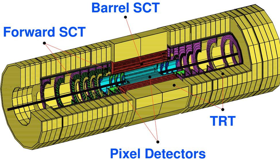
Figure 5.2: The ATLAS Inner Detector.
