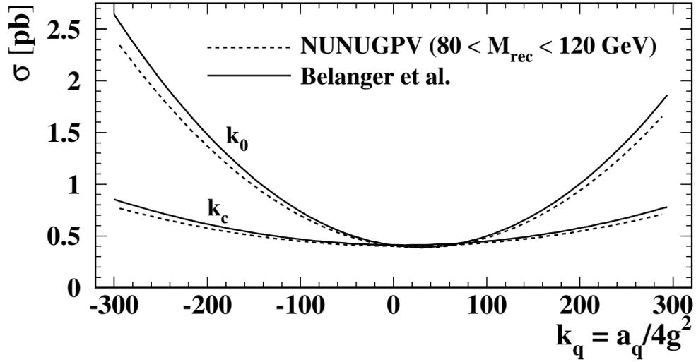
Figure 3.7: The cross-section for  $e^+e^- \rightarrow Z\gamma\gamma$  as a function of the anomalous couplings at the  $ZZ\gamma\gamma$  vertex, comparing the prediction of NUNUGPV with the results of Belanger *et al.* [24] at  $\sqrt{s} = 200$  GeV. The energy scale  $\Lambda = M_W$ . Cuts on the photons of  $E_\gamma > 5$  GeV and  $20^\circ < \theta_\gamma < 160^\circ$  were used.
