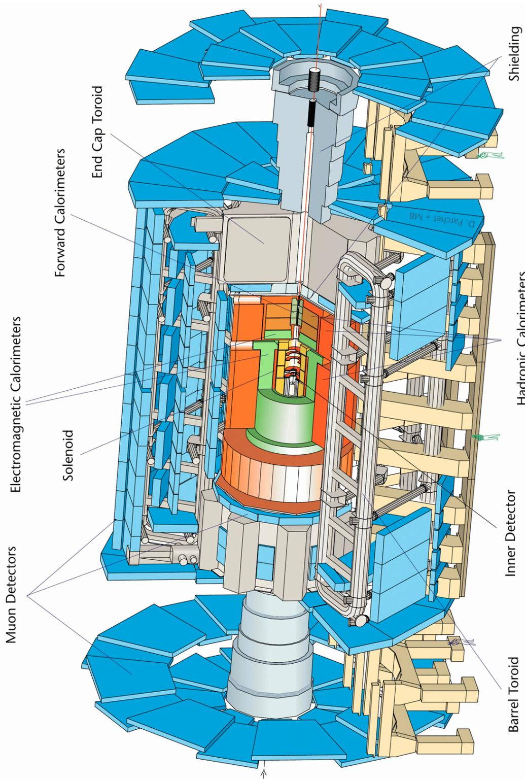
Figure 5.1: The complete ATLAS detector.
