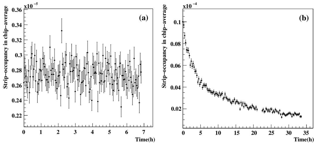
Figure 5.11: The typical noise occupancy values for one chip over a period of several hours with (a) and without (b) pre-biasing of the modules.
