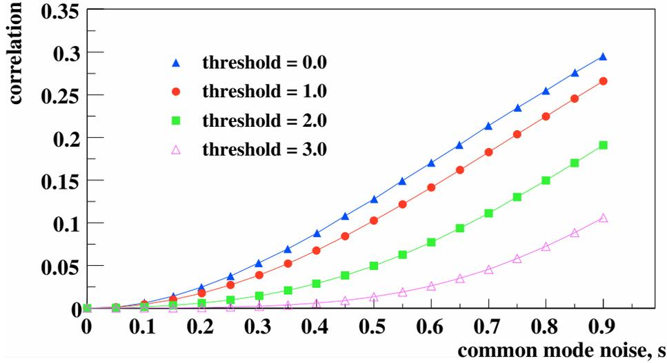
Figure 5.13: The correlation between two channels as a function of common-mode noise,  $s$ , for thresholds,  $\tau = 0, 1, 2, 3$ .
