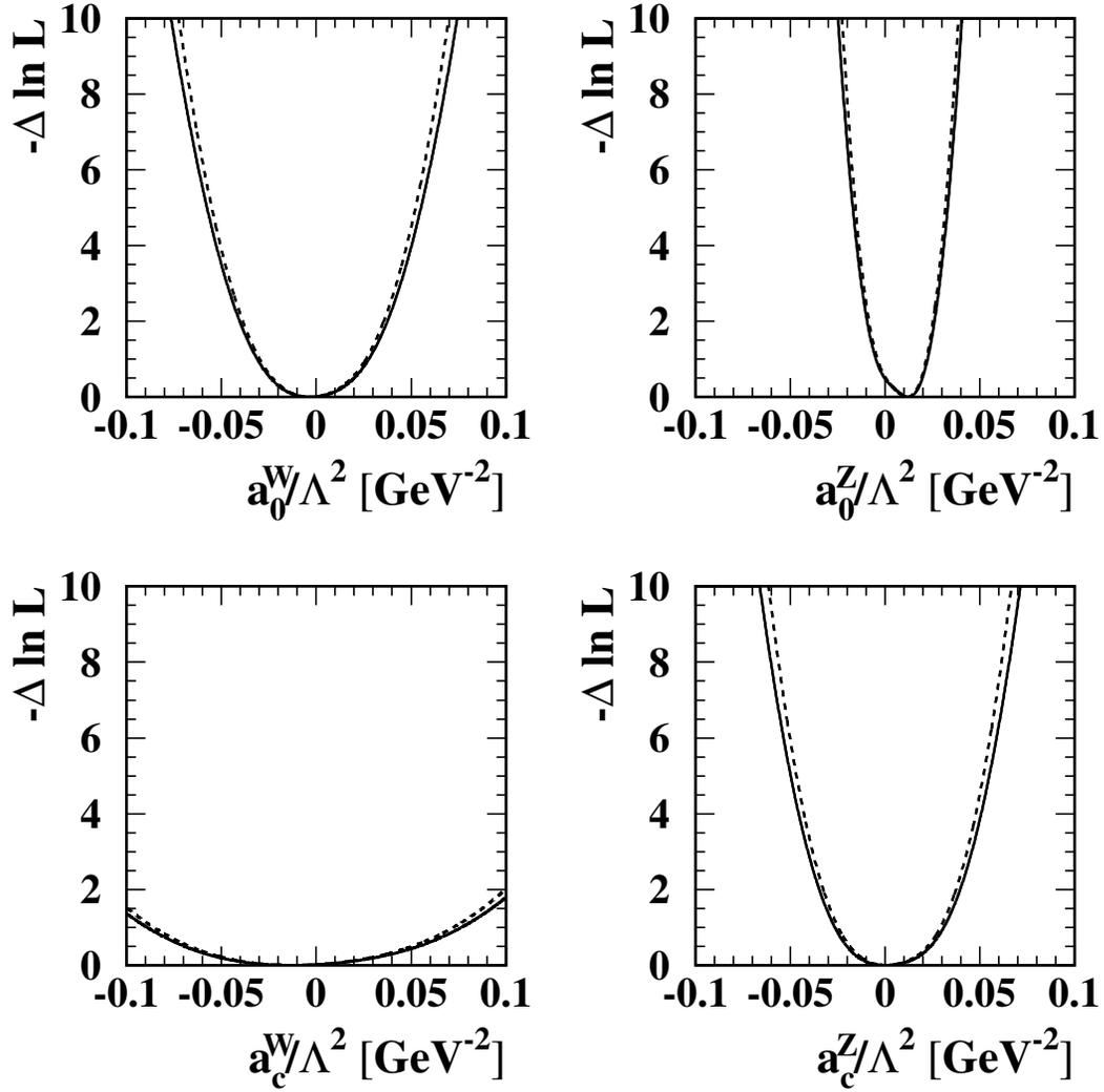
Figure 4.3: The one-dimensional likelihood curves for each of the anomalous coupling parameters from  $e^+e^- \rightarrow \nu\bar{\nu}\gamma\gamma$  with (solid line) and without (dashed line) the systematic uncertainties. The parameters not plotted are fixed at zero.
