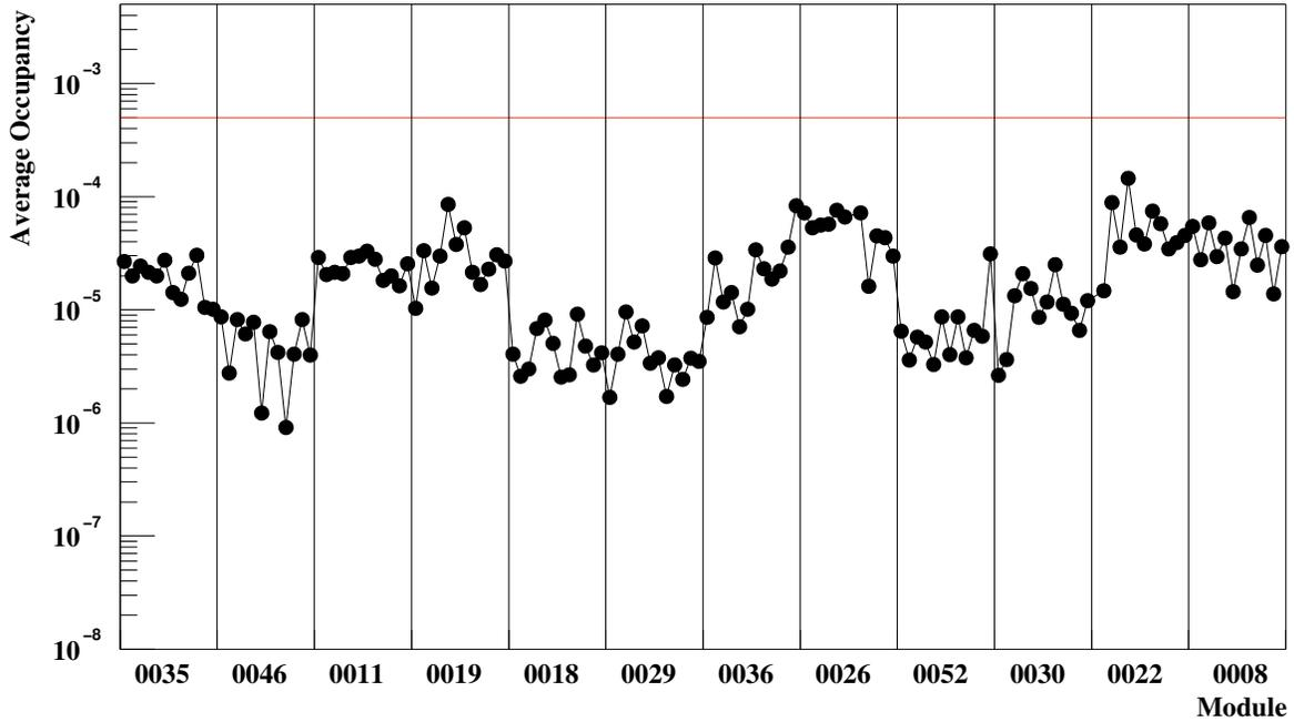
Figure 5.8: The noise occupancy values at 1 fC threshold by chip for a row of 12 modules on the sector, compared to the specified limit of  $5 \times 10^{-4}$ . The module names are given on the  $x$ -axis: the 12 points per module correspond to the chip averaged noise values.
