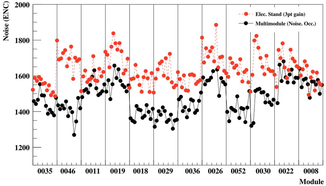
Figure 5.10: The ENC values by chip comparing between a row of 12 modules on the sector with their stand-alone performance, as derived from noise occupancy measurements. The module names are given on the  $x$ -axis: the 12 points per module correspond to the chip averaged values.
