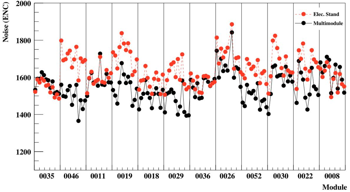
Figure 5.7: The ENC values by chip as derived from three point gain scans, comparing module performance in a row of 12 on the sector with their stand-alone performance. The module names are given on the  $x$ -axis: the 12 points per module correspond to the chip averaged noise values. The ENC values are in units of the electron charge.
