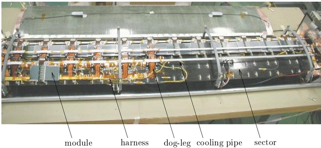
Figure 5.5: Photograph of the barrel system test populated with 13 modules, including one full row of 12
