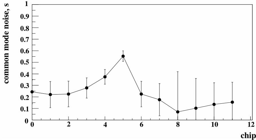
Figure 5.16: Common-mode noise by chip, obtained from the quadratic difference between the S-curve noise values  $Q_{\text{rnd}}$  (without noise injection) and  $Q_{\text{tot}}$  (with noise injection).
