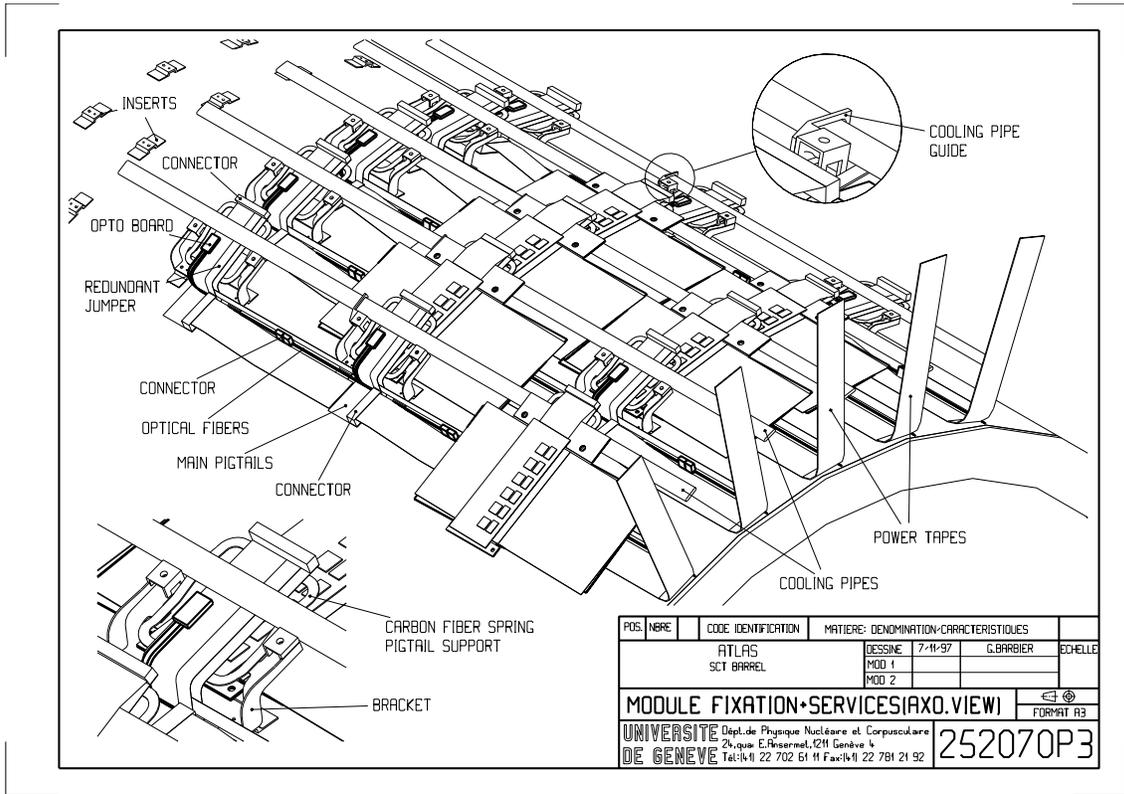
Figure 5.4: The design of an SCT barrel as used at the system test [86].
