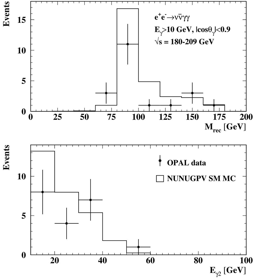
Figure 4.2: Recoil mass and second photon energy distributions for the accepted  $\nu\bar{\nu}\gamma\gamma$  events in OPAL data and Monte Carlo.
