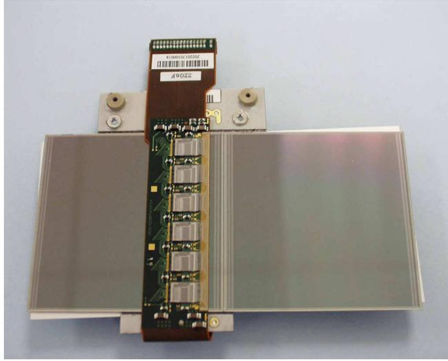
Figure 5.3: Photograph of a single SCT barrel module. The six chips on the upper side of the hybrid card are visible.
