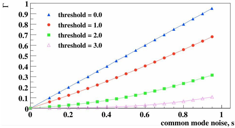
Figure 5.14: The observable  $\Gamma$  as a function of common-mode noise,  $s$ , for  $\tau = 0, 1, 2, 3$ .
