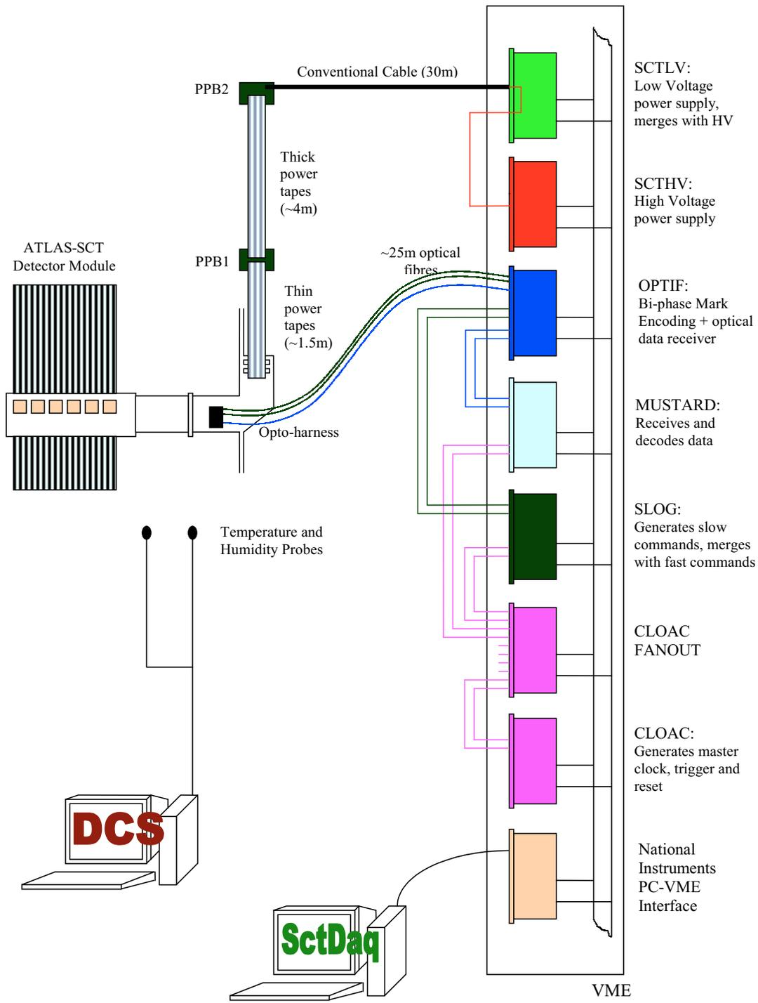
Figure 5.6: The system-test DAQ-system.
