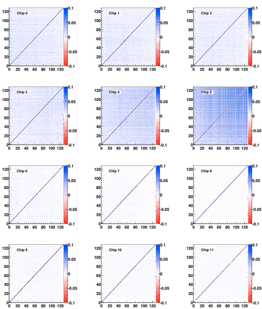
Figure 5.17: Correlation matrices seen with noise injection. The x- and y-axes indicate the channel number from 0 to 127 and the gray-scale shows the amount of correlation. It is evident that the greatest noise pick-up was seen by chip 5.
