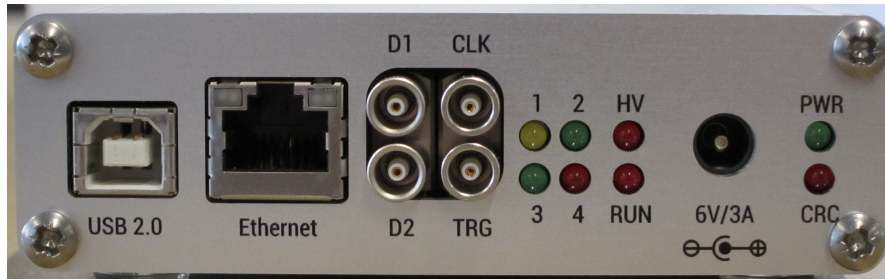
Figure 1: The DTB front panel featuring (from left to right) the USB2.0 port, the Gigabit Ethernet connector, the digital scope outputs D1 , D2 , the clock and trigger inputs, four status LEDs, the HV and detector power LED, the AC connector, and the DTB power and CRC LEDs.
