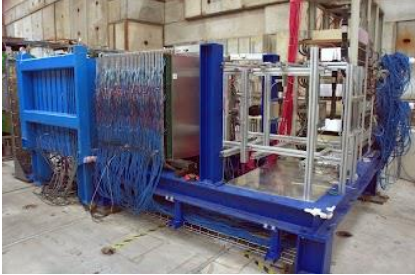
Figure 2. Photograph of the DHCAL setup at CERN showing the Main Stack with tungsten plates followed by the TCMT with steel plates.
