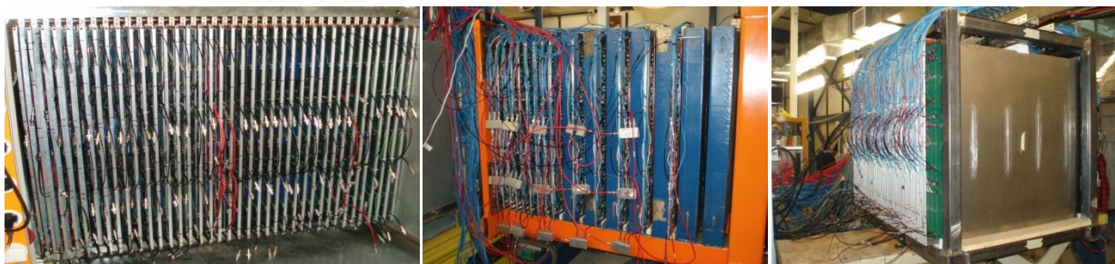
Figure 1. Left: The Main Stack (before cabling), middle: the TCMT, right: the 50-layer configuration with minimal absorber material.
