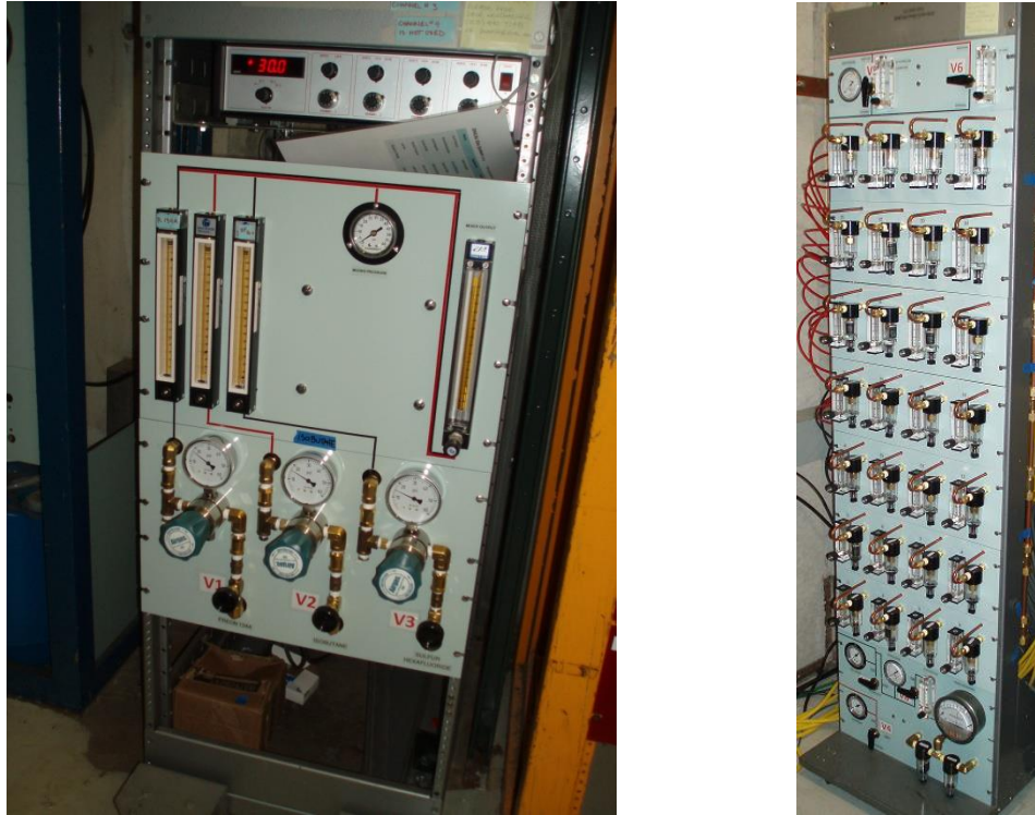
Figure 15. The DHCAL gas mixing system (left) and the gas distribution system (right).
