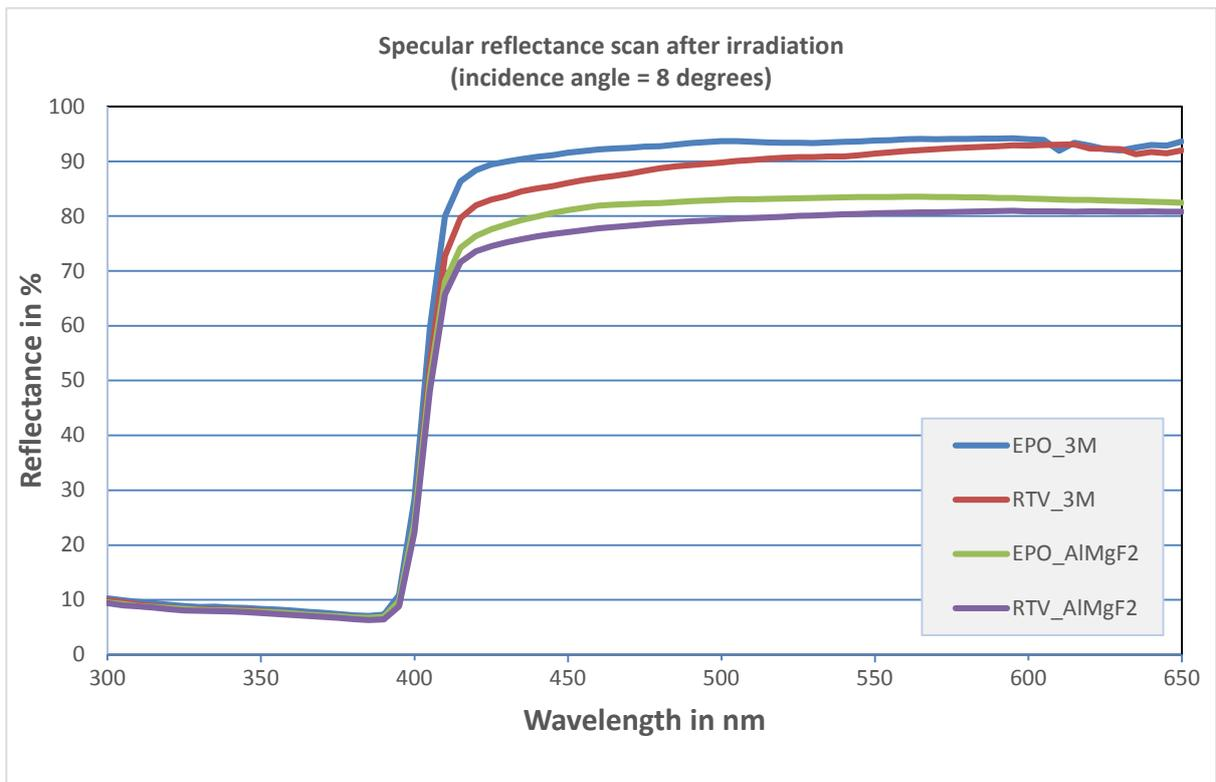
Figure 6: Specular reflectance of samples 1 – 4 after irradiation.
