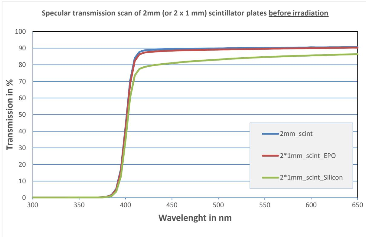
Figure 2: Specular transmission of the samples 1 – 3 versus wavelength, prior to the irradiation. The 5 – 10 % lower specular transmission of the RTV silicone glue is mainly due to the more diffuse aspect of this glue.
