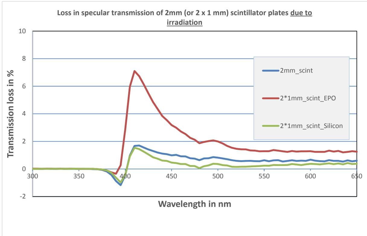
Figure 5: Loss of transmission due to the irradiation. The scintillator sample shows a very small loss of 1-2% close to the cut-off wavelength. The RTV glue does not lead to any additional transmission loss. The H301 glue shows a transmission loss of about 1% increasing to 7% close to the cut-off wavelength.
