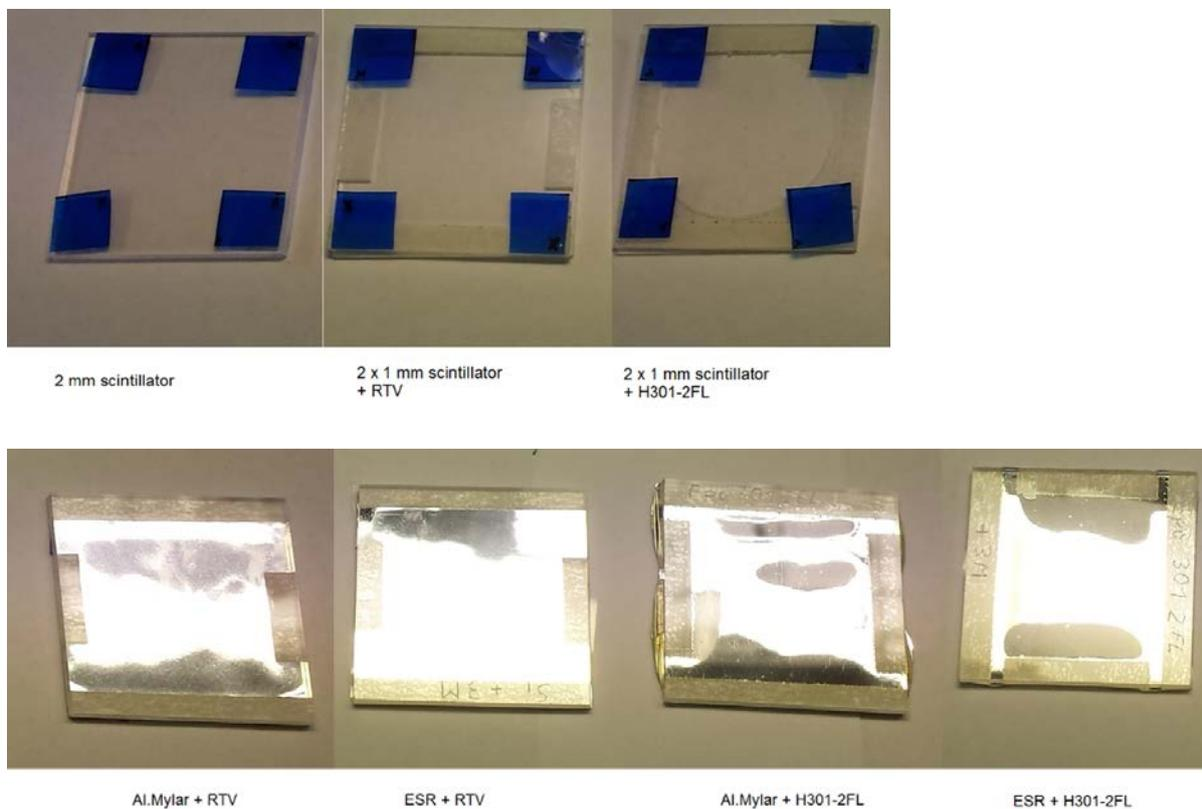
Figure 1: Photos of the seven samples, taken after the irradiation. The blue squares on the photos in the top row are remainders of the dosimetry film, which was used for an independent check of the dose and its uniformity (see sec. 4).
