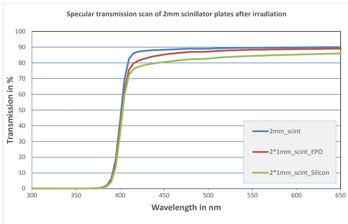
Figure 4: Post-irradiation measurement of the specular transmission of samples 1 – 3. Compared to Figure 2, one can note a slight reduction of the transmission of the Epotek glue sample.
