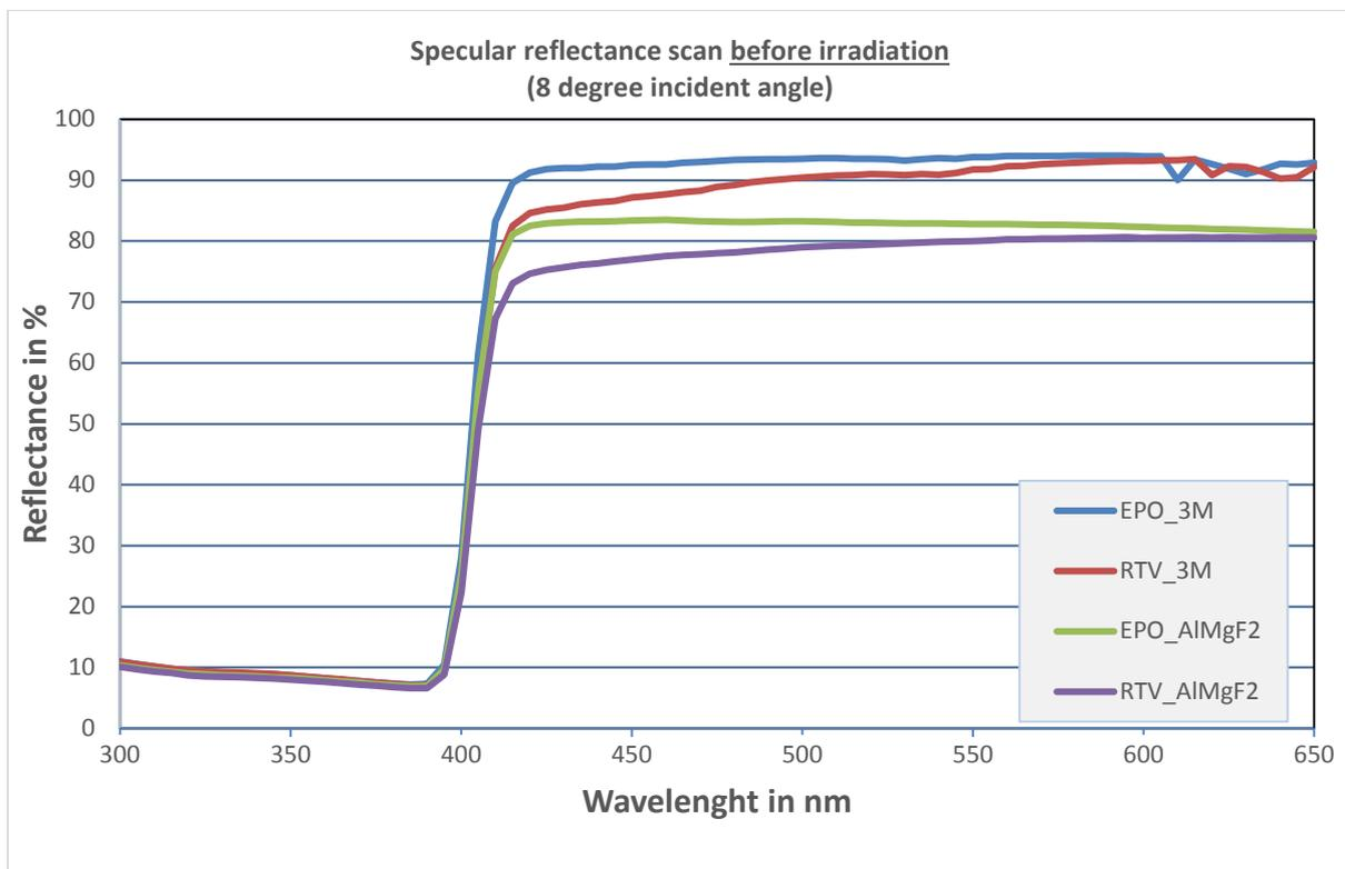
Figure 3: Specular reflectance of the samples 4 – 7 for an angle of incidence of 8°, prior to the irradiation.
