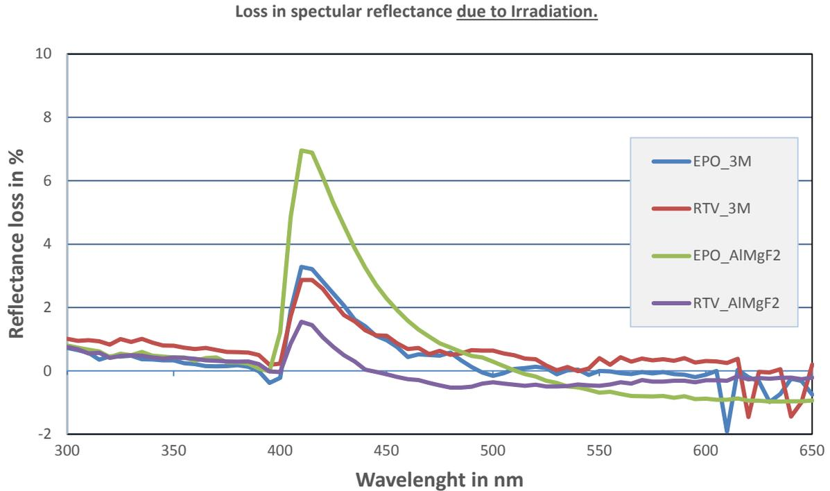
**Figure 7: Loss in specular reflectance of samples 4 – 7 due to irradiation. The two samples glued with Epotek H301 glue show maximum losses of 3 and 7%. The RTV glued samples show losses of 1.5 – 3%.**
