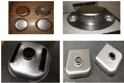
Figure 3 Stamped parts for the DQW (top) and RFD (bottom) at Niowave.
