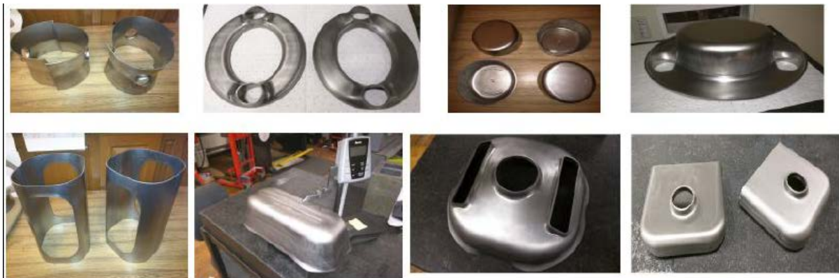
Figure 24: Stamped parts for the DQW (top) and RFD (bottom) at Niowave.
