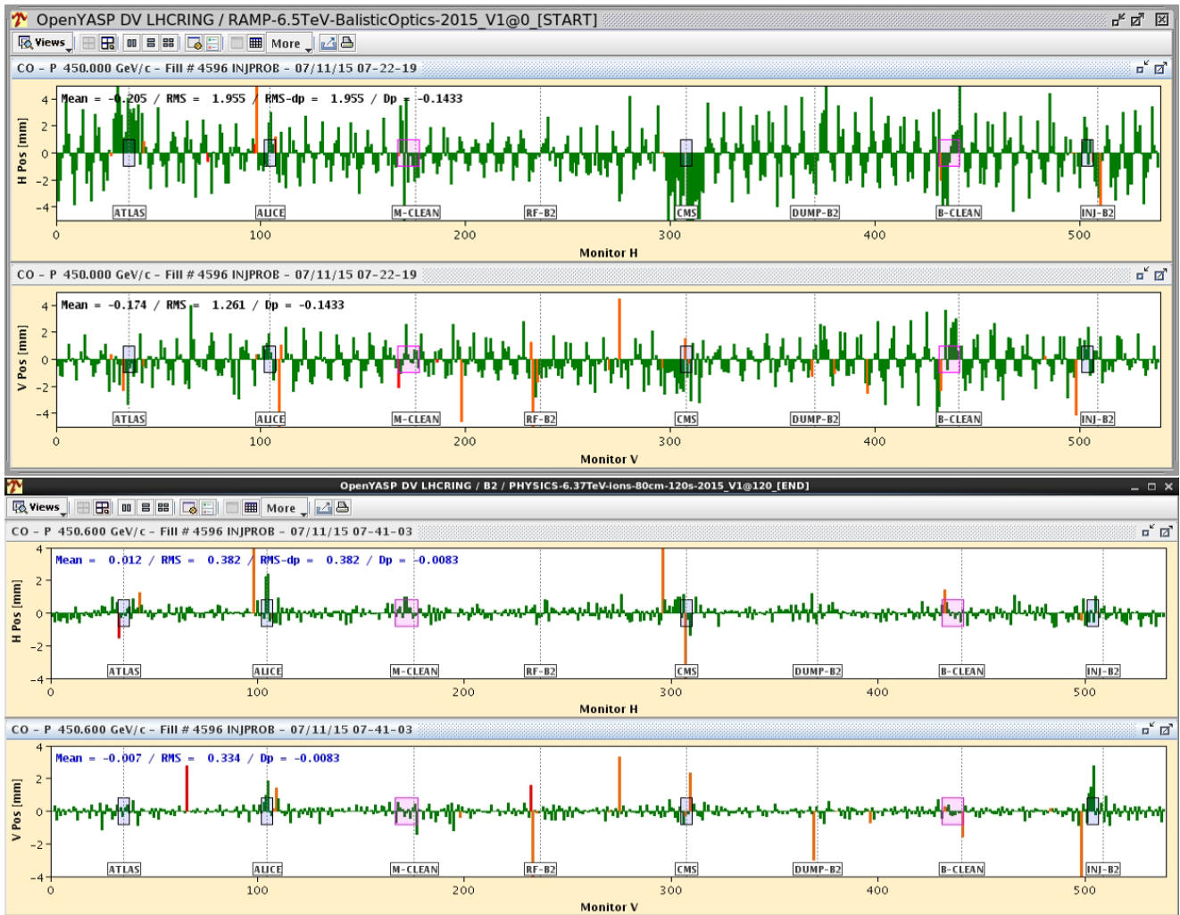
Figure 3: Raw beam 2 orbit after the first injection (before any correction, top) and after correction (bottom). The rms of the corrected orbit is very similar to the rms of the standard orbit (without the crossing and separation bumps).
