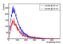
Figure 5. Pulse amplitude spectra for a candle placed at  $\sim$ 20 cm and  $\sim$ 30 cm distance from the detector with a charge preamplifier. The shape of the spectrum does not change, a clear indication for single electron pulses.
