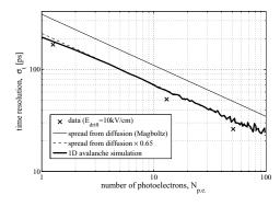
**Figure 8.** Dependence of the measured time resolution with the mean number of photoelectrons, for fixed amplification and drift fields. A resolution of 200 ps per single photoelectron and 27 ps for 50 photoelectrons has been achieved.
