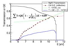
**Figure 2.** Transmission, refractive index of MgF<sub>2</sub> and quantum efficiency of CsI in reflective mode which were used for the calculation of the number of photoelectrons.
