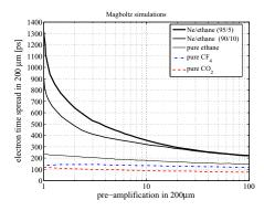
**Figure 3.** Electron time spread due to diffusion for several gases as a function of the achieved pre-amplification in a 200  $\mu$ m gap.
