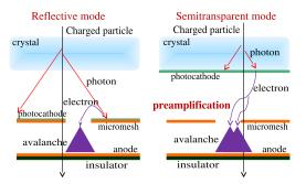
**Figure 1.** Schematic view of the charged particle detection principle, in the two modes; Reflective mode: a thin CsI layer is deposited on top of the micromesh; Semitransparent mode: CsI is deposited on the bottom surface of the UV crystal, defining a drift gap with the micromesh.
