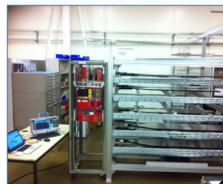
Figure 5. Cosmic stand at CERN for the final quality control of GE1/1 superchambers.
