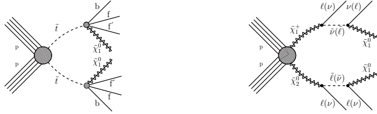
Figure 1: Signal models for top squark pair production with subsequent four-body decays (left), and chargino-neutralino pair production with decays via sleptons and sneutrinos (right). Antiparticle labels are suppressed. The ISR jet used in the analysis is not shown in these diagrams.
