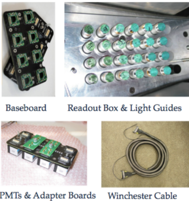
Fig. 2. Pictures of the base board, the readout box with light guides, PMTs and adapter boards, and the Winchester cable as examples of the key components of the upgrade.
