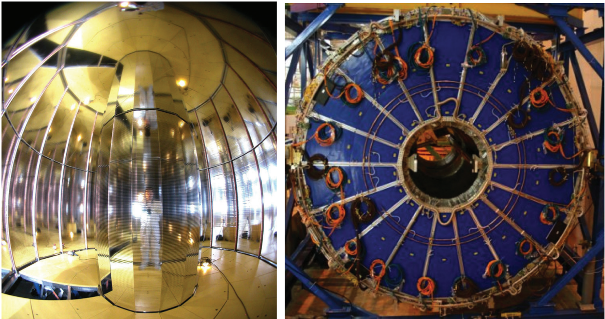
Figure 1: Left: Fish-eye view of the TPC field cage during assembly. The central high voltage electrode is located at the top of the image and reflects like a mirror. Right: The two endplates of the TPC are divided into 18 sectors holding two readout chambers (ROC) each. The ROCs and front-end electronics are hidden behind the blue covers.
