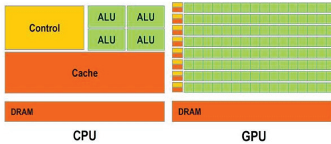
Fig. 1. CPU and GPU: different distributions of resources.
