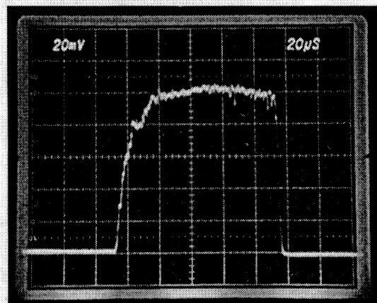
Fig. 5 RFQ2 output beam (vertical scale: 40 mA/div)
