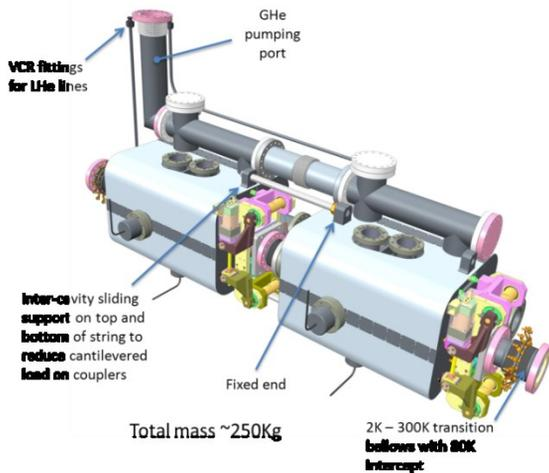
Figure 5: A string consisting of two dressed cavities with modified Saclay-II tuners.
