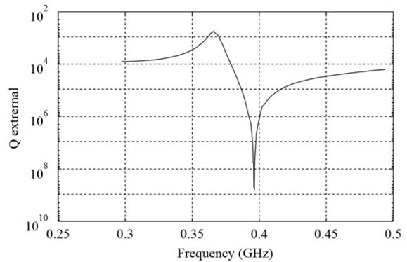
Figure 4: Q factor of the LOM coupler connected to a quarter wave resonator simulated in CST.
