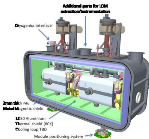
Figure 6: Side loaded cryomodule with full access to internal components after assembly and installation.
