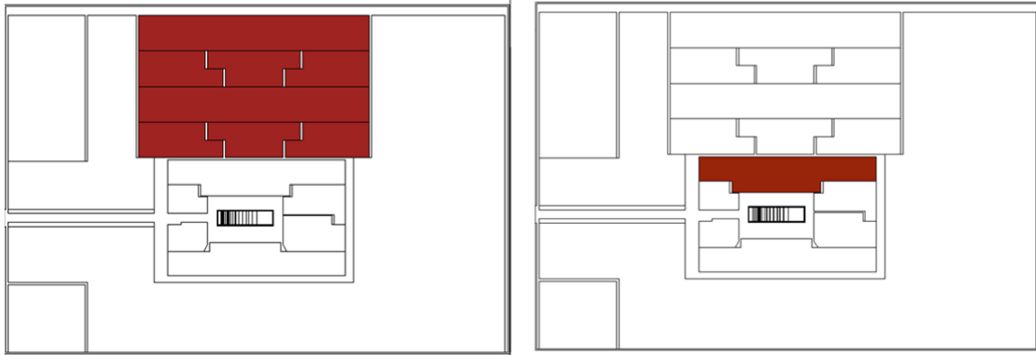
Figure 15: Outer (left) and inner (right) removable cast iron shielding in the SHiP target area, whose residual dose rates were evaluated standalone.
