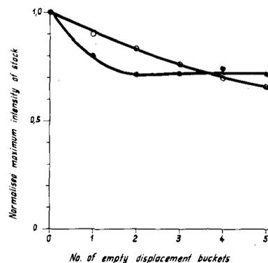
Fig. 8 - Intensity of stacked beam as a function of the number of empty displacement buckets passed through the stack.
