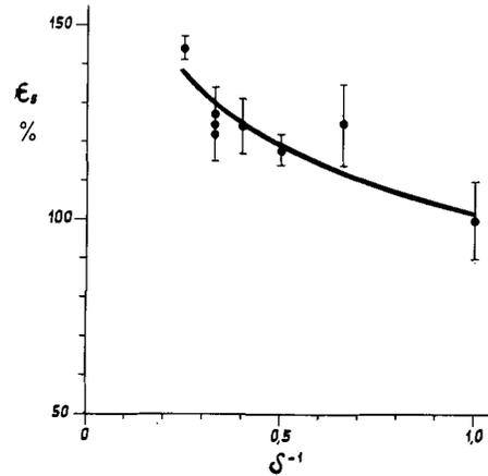
Fig. 6 - Stacking efficiency as a function of emptiness of bucket ( $\Gamma = 0.2$ ;  $5 < n \leq 10$ ,  $n =$  number of pulses stacked).
