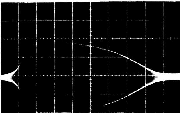
Fig. 3 - Typical signal from the electrostatic pickup electrode when a 40-pulse stack is scanned by an empty bucket. The high energy end of the stack is on the left.
