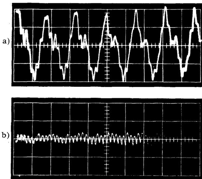
Fig. 9 - a) Van de Graaff terminal voltage ripple, without stabilisation (Sensitivity: 1 div. = 500 V; Time-base: 1 div. = 0.1 sec).
