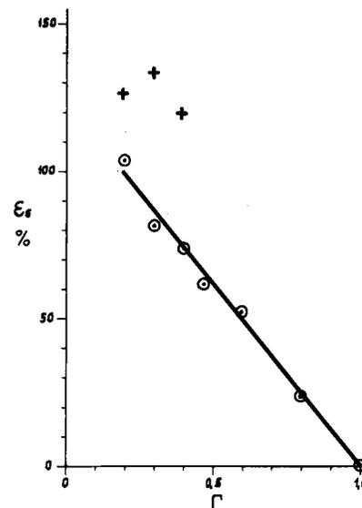
Fig. 4 - Stacking efficiency as a function of stable phase parameter ( $2 < n \leq 10$ ,  $n$  = number of pulses stacked).
