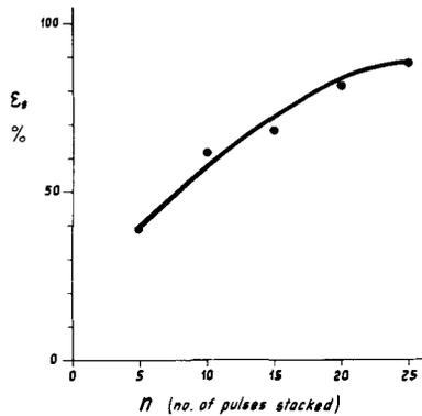
Fig. 5 - Stacking efficiency as a function of number of pulses stacked (Full buckets;  $\Gamma = 0.46$ ).
