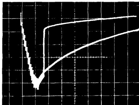
Fig. 10 - The figure shows the accumulation of 12 pulses and their subsequent decay due to gas scattering. The vertical scale is 0.4 mA per division, and the horizontal scale 0.2 sec per division. The upper trace shows the instability that occurs without clearing fields, and the lower trace the normal decay with 4 V applied to the clearing field electrodes.
