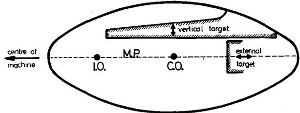
Fig. 2 - Vacuum chamber cross section — I.O.: Injection orbit; C.O.: Central orbit; M.P.: Median plane.
