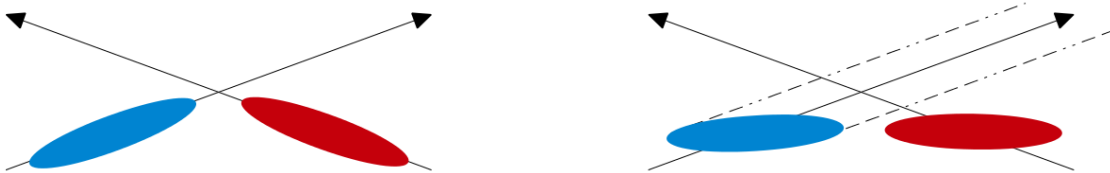
Figure 1: Bunches colliding with a crossing angle without (left) and with (right) the crab crossing.
