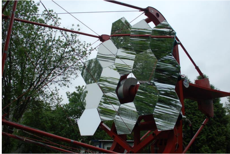
Figure 7 Pre-integrated SST-1M optical system with telescope structure. Three remaining mirrors on the bottom of the telescope are plan to be integrated in autumn 2015.
