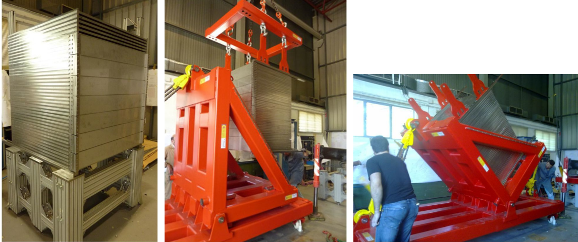
Figure 30: Left: Mechanical structure almost finished. Center: Mechanical structure being placed on the rotation tool. Right: Mechanical structure during the rotation from horizontal to vertical position.
