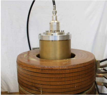
Figure 3: Measurement set-up: Sample holder in solenoid.
