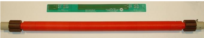
Fig.2. The Printed Circuit Board (PCB) with both 26-mm and 130-mm long, 28 mm in diameter probes (top) and PCB probe holder (bottom). Typical probe rotational speed is 1 Hz.
