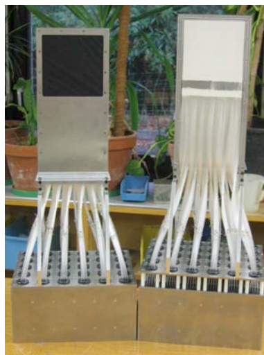
Fig. 4.6 New SFD X and Y planes under construction
