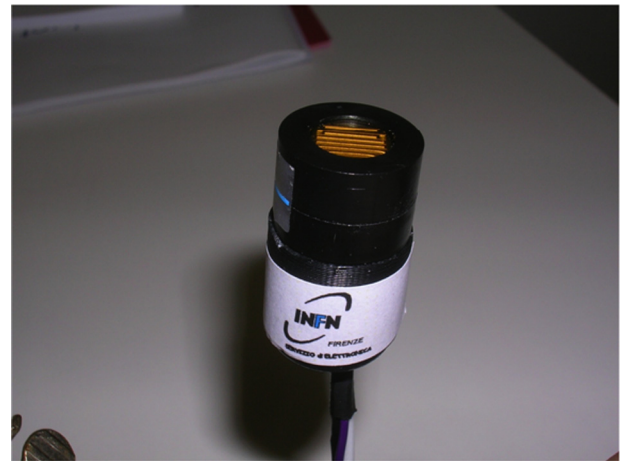
Fig. 2. The HAMAMATSU R7400 U-03 photomultiplier connected to the custom made divider.
