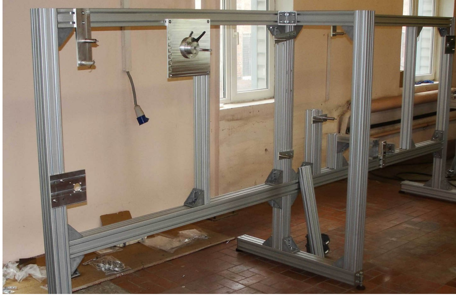
Figure 6: Mechanical frame of the scanner at Kurchatov institute currently under construction
