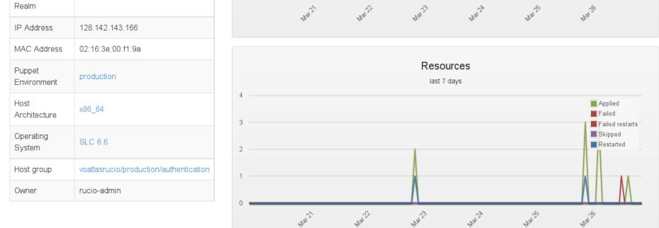
Configuration of the nodes is done via Puppet, a declarative client/server management system. A Ruby-like language describes which software should and should not be installed, and how it must be configured. Puppet will ensure that this configuration is enforced at all times.
