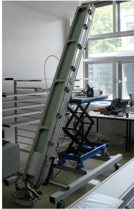
Figure 3.16: Step 9: Filling of glue into casting jig
