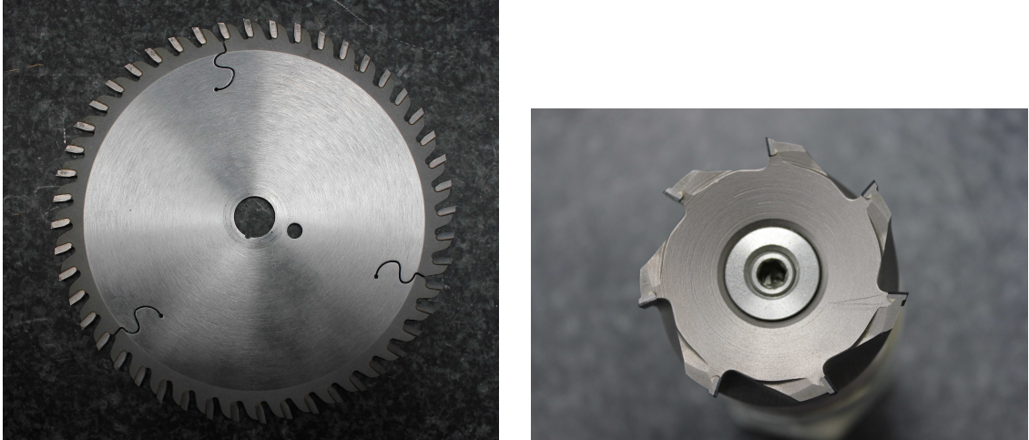
Figure 3.21: Tools: Saw blade for pre-cut (left) and a diamond head for final optical cut (right).
