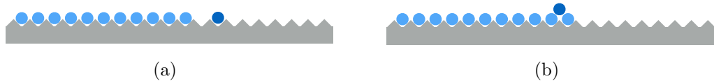
Figure 3.38: Two different defects which can occur during the winding process. In (a) the current fibre jumped in the wrong thread and leave an empty space. (b) shows a fibre lying in the wrong layer.
