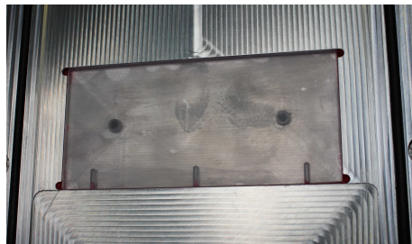
Figure 3.15: Step 5: Placing of endpiece on readout side (left) and mirror side (right) in casting mold and sealed with Latex
