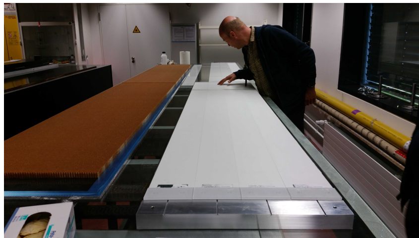
Figure 4.5: A photo of seven of eight dummy mats with endpieces which have been placed in the template. The 5 m honeycomb panel is visible on the left. The grooves in the template are visible and continue under the mats.
