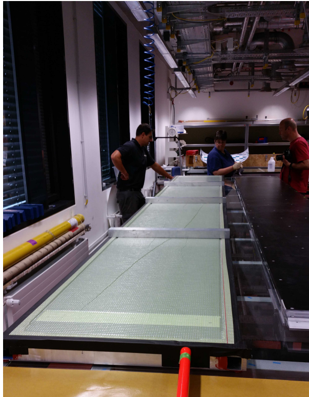
Figure 4.18: The vacuum press assembly overtop of the panel during the first pressing step.
