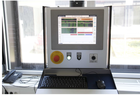
Figure 3.4: Control panel of the winding machine.
