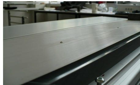
Figure 3.14: Step 2: Preparation of fibre mat with spacing lines
