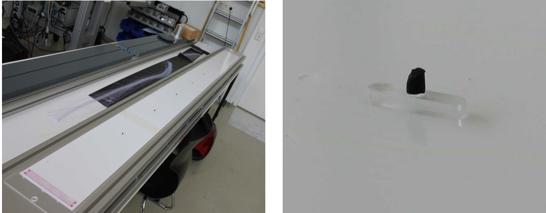
Figure 3.18: Optimization of casting process parameters: Casted dummy with EPOTEK 301, zoomed view of one alignment pin.
