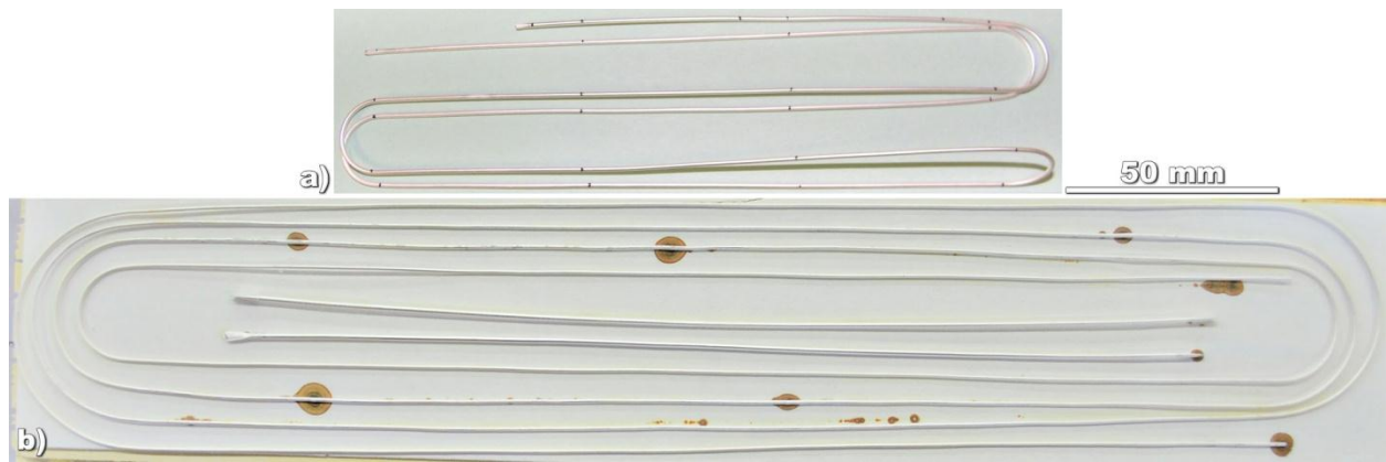
Figure 1. Digital camera images of (a) the 1 m open-ended wire and (b) the 2.4 m open-ended wire with two shorter, open-ended straight samples placed in the middle of the hair pin. The dark dots on the 1 m wire in (a) are added marks used to define the cutting into short straight sections. In (b) brown stains are seen on the alumina fiber sheet under the strand where leaks generated by internal pressure have occurred during heat treatment. Both large individual leaks and clusters of smaller clusters can be observed on the straight sections of the 2.4 wire.
