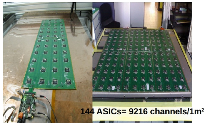
Fig. 2. Development of electronic readout for a large GRPC: size of 1 m 2 .
