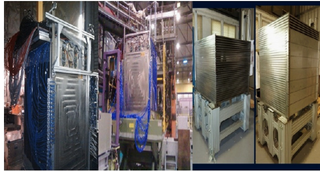
Fig. 4. Construction of the SDHCAL prototype 460 800 electronics channels and self-supporting mechanical structure 50 working with power-pulsing.
