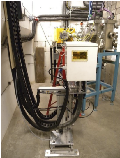
Figure 2: The pre-configured XY-axis Cartesian robot system and cool box within the high intensity irradiation area at the Medical Physics MC40 cyclotron, University of Birmingham
